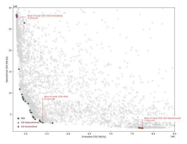
Figure 21: Results of the multi- (MO - green dot) and single-objective (SO-operational - red triangle, SO-operational - purple cross) optimizations on the objective space for cumulative energy demand (heating energy carrier: gas). Source: (Kiss & Szalay, 2020).
