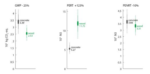
Figure 8: Contribution Analysis and comparison of concrete and timber structure. Source: (Schneider-Marin et al., 2020).
