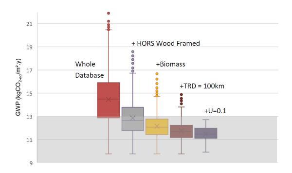
Figure 23: Distribution of the GWP impacts of the full database (left), and other subpopulations with cumulative constraints by the sensitivity indices of the design parameters. The grey zone represents GWP impacts below the SIA2040 objective. GWP axis starts at 9 kg CO2- $eq/m_2$ .y.
