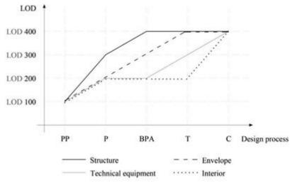
Figure 6: Design process and LODs for different construction categories. (PP) Project Planning, (P) Project, (BPA) Building Permit Application, (T) Tendering and (C) Construction. Source: (Cavalliere et al., 2019).
