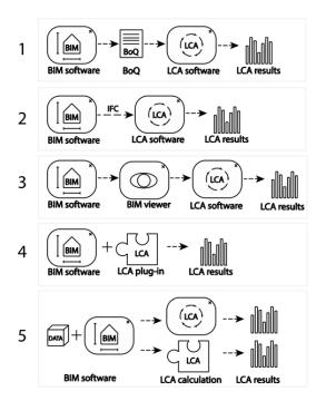
Figure 13: Different BIM-LCA approaches. Source: (Wastiels & Decuypere, 2019).
