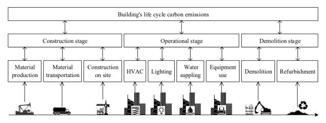
Figure 15: Schema of Boundary of Building's Life Cycle Carbon Emissions (BLCCE) approach. Source: Lu, Kun et al.
