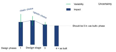
Figure 3: Qualitative representation of the development of environmental impacts and the variability during the design process form the early stage 1 to the final as-built stage 4.
