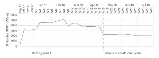
Figure 19: Evolution of total results for embodied GWP in t CO<sub>2</sub>-e throughout the design process. Source: (Hollberg, Genova, et al., 2020).
