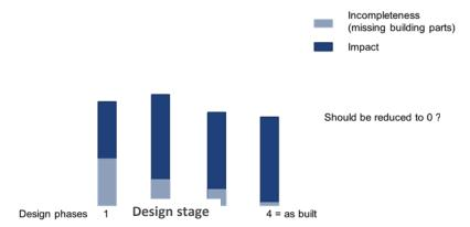
Figure 4: Qualitative representation of the development of environmental impacts and incomplete data (missing building parts) during the design process form the early stage 1 to the final as-built stage 4. In the LCA done as built there are still parts that are usually not considered as its expected they have a minor contribution to final LCA results.
