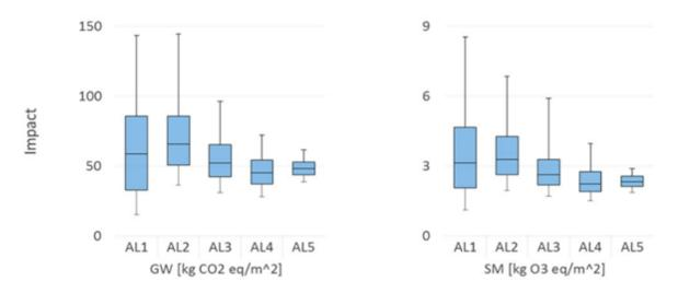
Figure 11: Probabilistic distributions of impact metrics (Global warming, Smog creation) for an ICF wall. AL1 to 5 = Assembly level 1 to 5. CV = Coefficient of variation. MAD-COV = median absolute coefficient of variation Source: (Tecchio et al., 2019).
