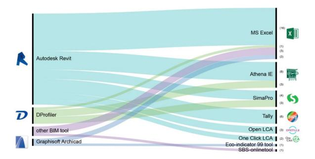
Figure 6: Software adoption in the selected cases studies; the coloured flow lines indicate the relationships between tools in data exporting from the BIM model to LCA analysis; on the left side, the chart gives evidence of the widespread adoption of Autodesk Revit (more than 80%) for BIM models; on the right side, the LCA tools are listed, counting in brackets the number of cases linked to each BIM software. Source: (Mora et al., 2020).
