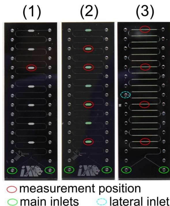
Figure 3.5 Different types of microreactors. Microreactor 1 contained 7 chambers each containing a sensor spot with a diameter of 100  $\mu\text{m}$ , 200  $\mu\text{m}$  or 300  $\mu\text{m}$ . In microreactor 2 the chambers were fully covered by oxygen sensors and microreactor 3 contained the oxygen sensor along the straight microfluidic structures of the channels.
