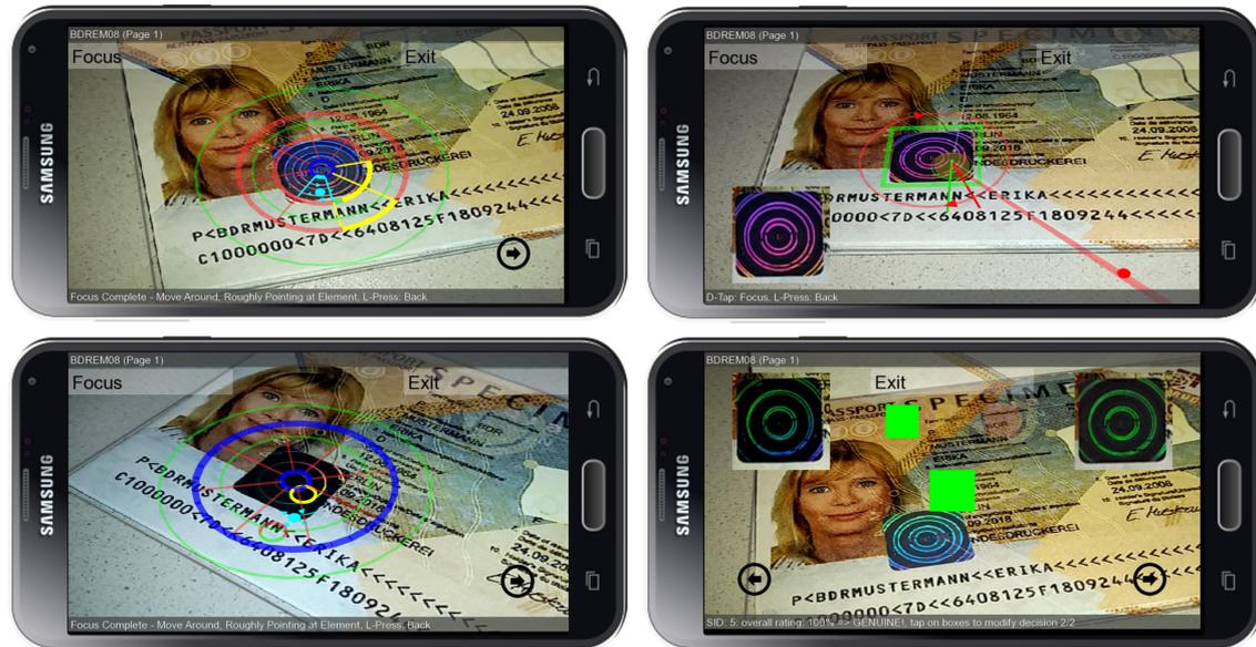
**Figure 6.16:** User interfaces for hologram verification: Constrained navigation (top-left), alignment (top-right) and hybrid user interfaces (bottom-left) are designed, implemented and evaluated within a user study. They allow to reliably capture image data suitable for automatic verification. Results are presented to the user in a summary (bottom-right).
