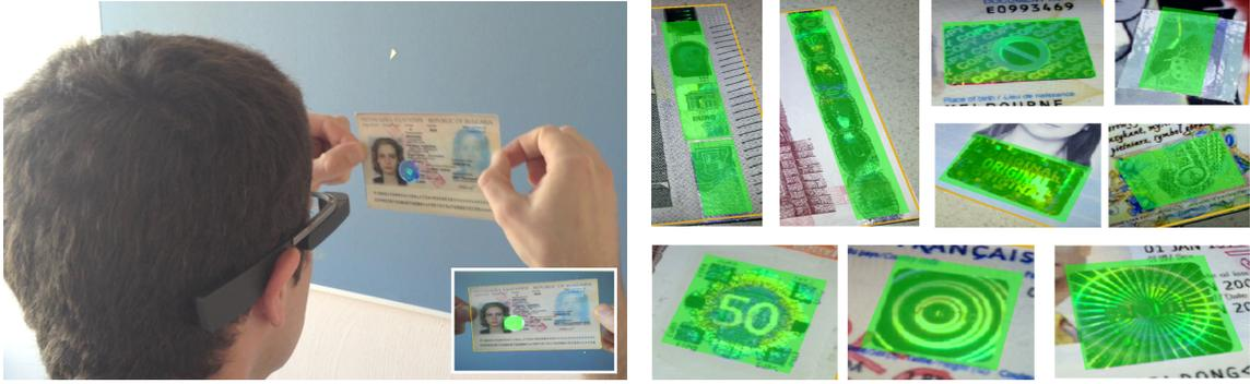
**Figure 5.4:** Left: Using Google Glass to perform hologram detection on a foreign passport. The picture as seen by the user is depicted in the inlay in the lower right corner. Right: Visualization of exemplary detection results in our prototype. Note that this is based on an approximation of the hologram region by a bounding rectangle, although we obtain a more detailed estimate of the region.
