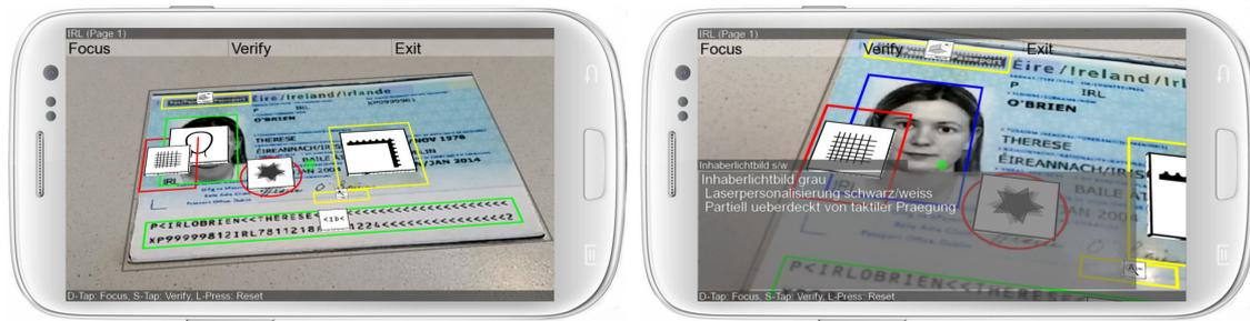
**Figure 5.13:** Mobile document verification system tracking a sample instance of the data page used in passport. The position of security features is augmented directly onto the document (left). Detailed information about an element can be triggered by pointing the camera at it (right).
