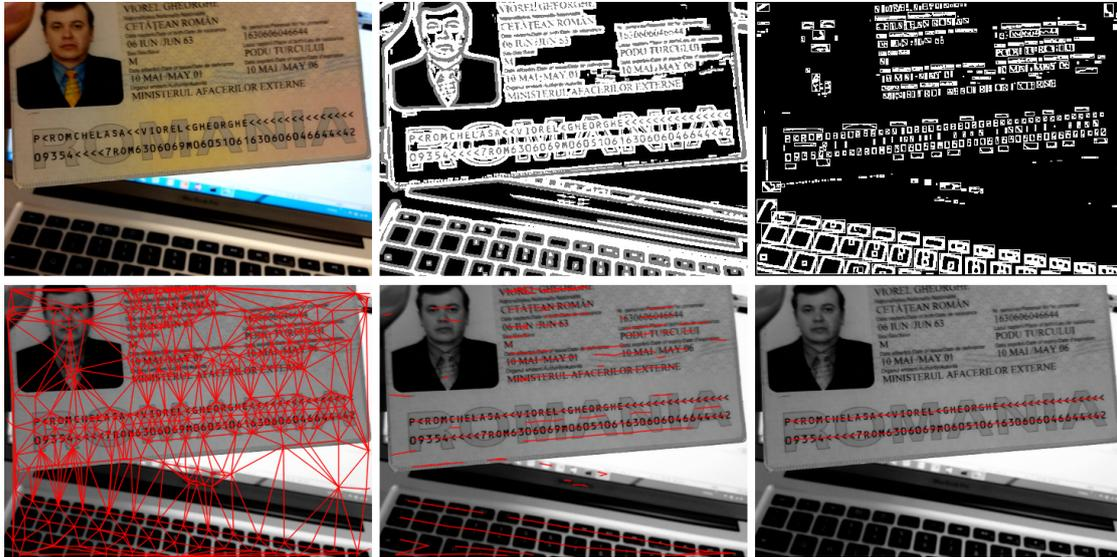
**Figure 4.4:** Steps in our algorithm. Top row: Input-image, segmentation result, filtered connected components. Bottom row: Delaunay triangulation, filtered pairs, final MRZ detection result.
