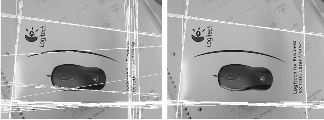
**Figure 3.4:** Influence of filtering text-like structures on line detection: Result on plain edge map (left). Result on filtered edge map (right).
