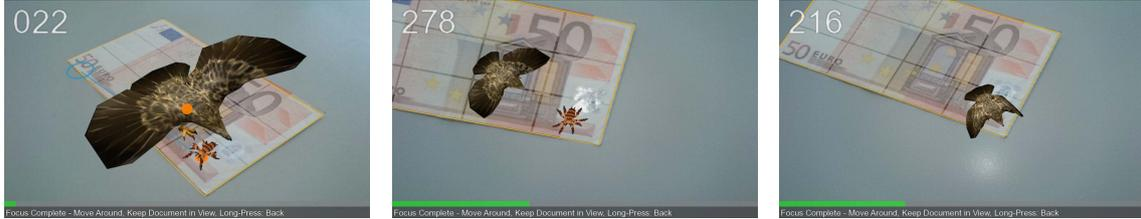
**Figure 5.8:** Screenshots from the game taken on the mobile phone. The eagle is circling over the target, on which the system places animated prey. By placing prey it suggests a new viewing position the user should reach with the mobile device to make the eagle attack and score.
