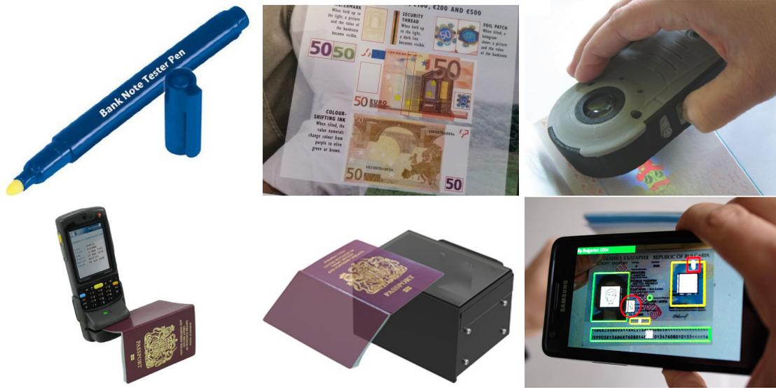
**Figure 1.2:** Exemplary tools for document inspection (left to right, top to bottom): Banknote Pen (<http://www.amazon.co.uk>), Manual (<https://www.ecb.europa.eu>), Doculus Lumus (Magnifying Glass, LEDs (White, UV), NFC Reader - <http://www.doculuslumus.com>), handheld and Passport Readers (<http://www.access-is.com>), Smartphone
