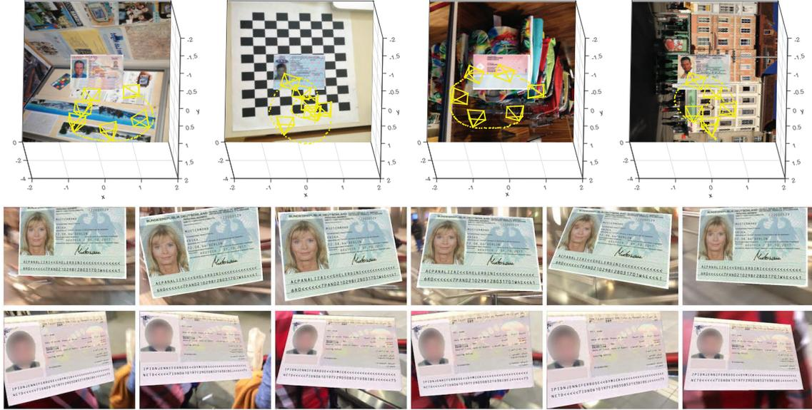
**Figure 4.8:** Top: Sequences of frames rendered onto a random background, and the corresponding camera trajectory. For better visibility, only every 25<sup>th</sup> frame is drawn as a frustum. Bottom: Sample frames from two sequences. As the document is rendered into a video, the background changes with each frame.
