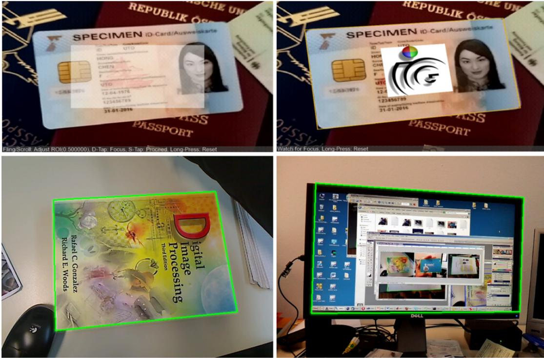
**Figure 3.2:** Top row: Visualization of the region of interest and tracking of the detected and rectified document region within a Mobile AR prototype. Bottom row: Since no assumptions about the contents of the region are made, the proposed approach has several other use cases.
