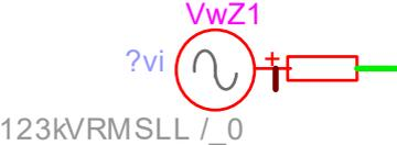
Figure 5.3.19. EMTP – RV block for substation modelled as the voltage sources with a Thevenin impedance
