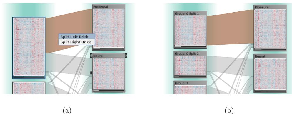
**Figure 7.5:** Split operation based on the ribbons between three bricks. (a) The split operation is triggered using the context menu of a ribbon connecting two bricks. (b) After the split operation the chosen brick was split into two bricks: The first contains all records the two bricks that were connected by the chosen ribbon share, while the second contains all others.
