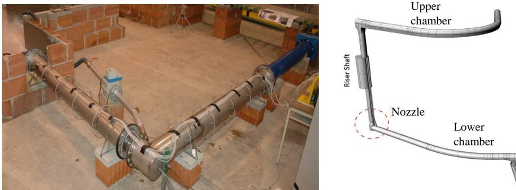
Figure 119: Burgstall surge tank, Left: Physical model, Right: 3D view [99]
