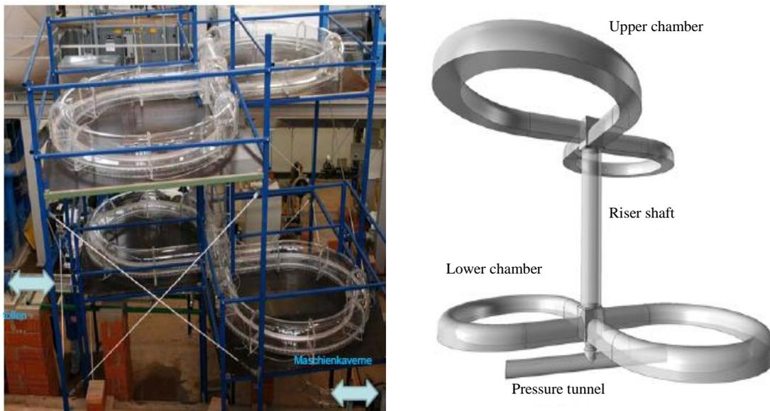
Figure 120: Physical model setup (left) and 3D view of surge tank (right) [100]
