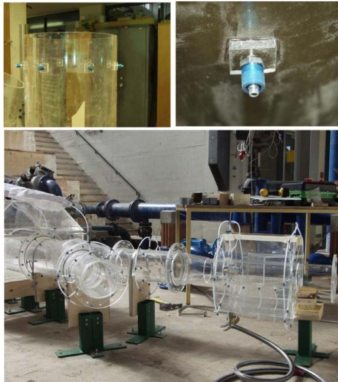
Figure 10: Control section and the pressure hole, Top: example of pressure hole, Bottom: picture of the ring line [26]
