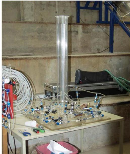
Figure 11: Pressure head calibration tool [26]
