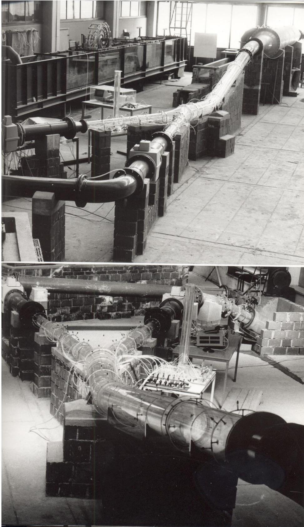
Figure A2: Installation of Y-bifurcator Alberschwende [40]
