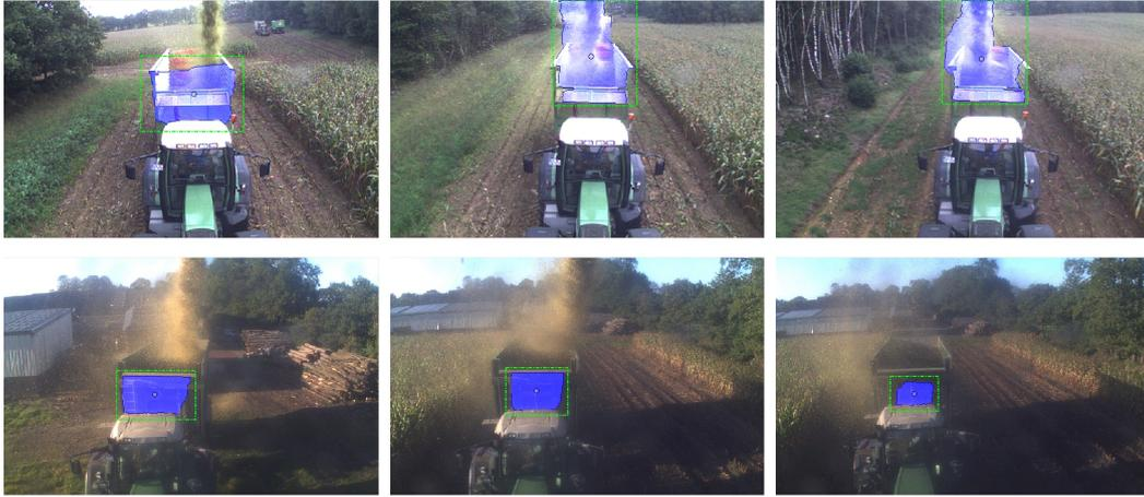
Figure 6.18: **Segmentation Failures in Agricultural Outdoor Environments:** Similar foreground background colors or blurry and homogeneous regions result in either over- or under-segmentation results. Although, the hanger is tracked correctly, the intermediate segmentations are not convenient and satisfactory.
