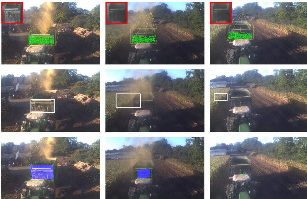
Figure 5.1: **Tracking in Harsh Outdoor Environments:** Appearance based template tracking (upper row) outperforms visual tracking decomposition [73] (middle row) and a Hough-based tracking approach [45] (bottom row) which are state of the art tracking methods. Both approaches are prone to fail as they cannot cope with the significantly large amounts of visible noise.
