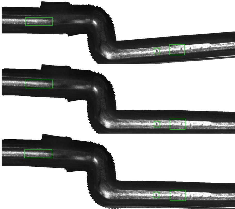
Figure 7.12: **Global Panorama Refinement Results:** The incrementally generated weld seam panorama (top) exhibits cumulative registration errors, which are corrected using graph based pose optimization (middle). The resulting image artifacts are finally removed by applying a global iterative alignment that minimizes feature point re-projection errors (bottom). [75]
