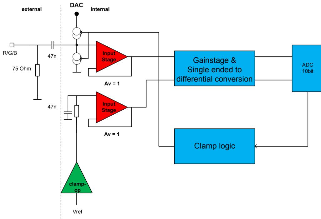
Figure 1.1: Principle Analog Video Frontend
