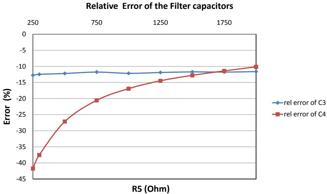
Figure 3.28: Relative error of the filter capacitors depending on R3 for correction of the op-amp
