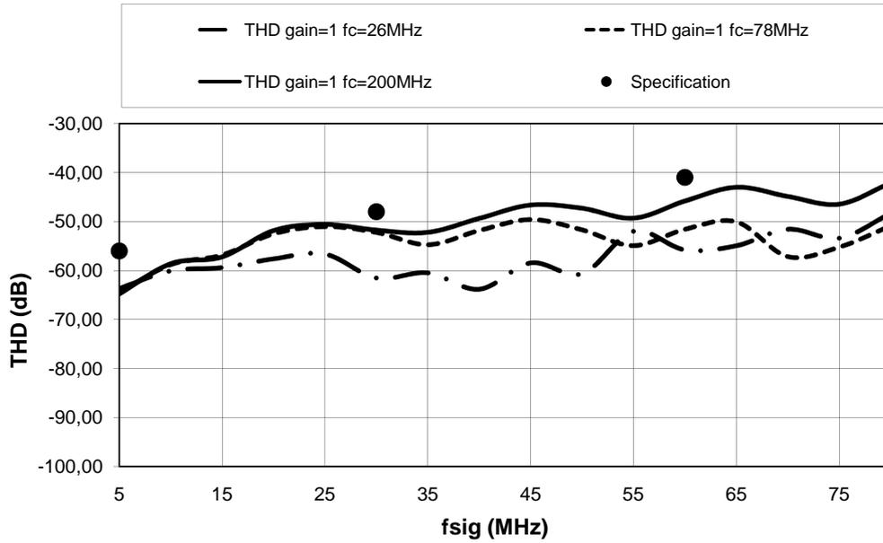
Figure 3.43: THD of the pre-processing at  $f_{\text{strobe}}=165\text{MHz}$  depending on the signal frequency
