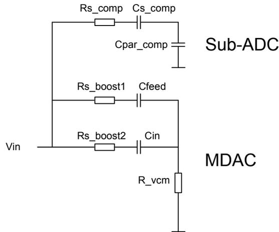
Figure 4.5: Sample network of sub-ADC and MDAC
