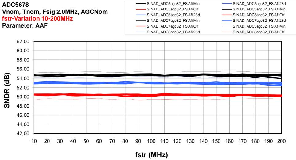
Figure 6.3: SINDR of the HD channels depending on fstroke
