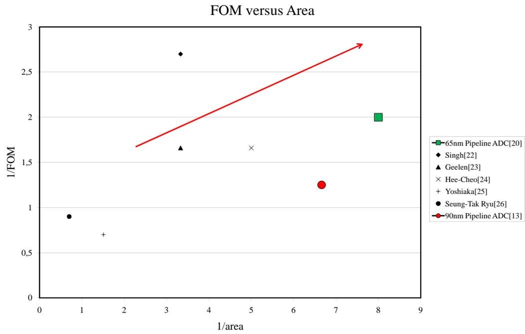
Figure 7.1:  $1/\text{FOM}$  versus  $1/\text{area}$  of the 65nm and 90nm pipeline ADC compared to state of the art ADCs
