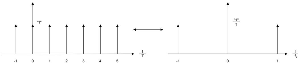
Figure 2.6: Transformation between time and frequency domain for the sampling function
