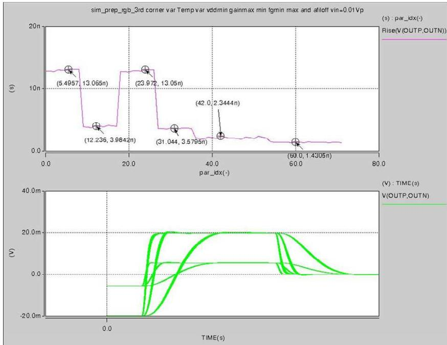
Figure 3.46: Rise time depending on the filter settings and process corners
