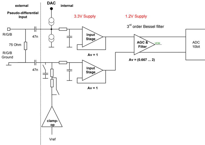
Figure 3.4: Principle Analog video Frontend with a 3<sup>rd</sup> order Bessel filter and only 2 stages
