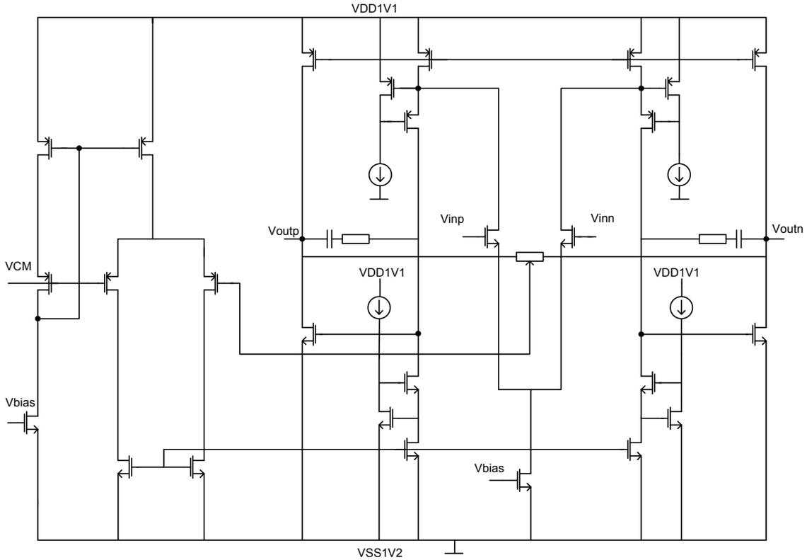
Figure 3.21: Topology of the AGC folded cascode op-amp
