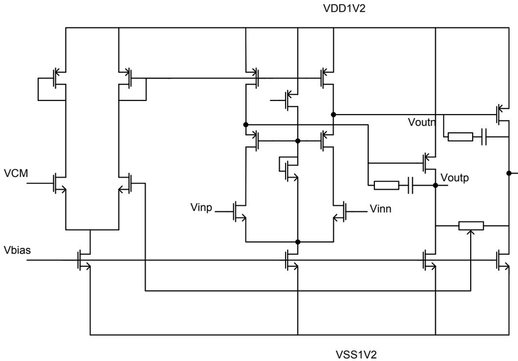
Figure 3.29: Op-amp of the first filter stage
