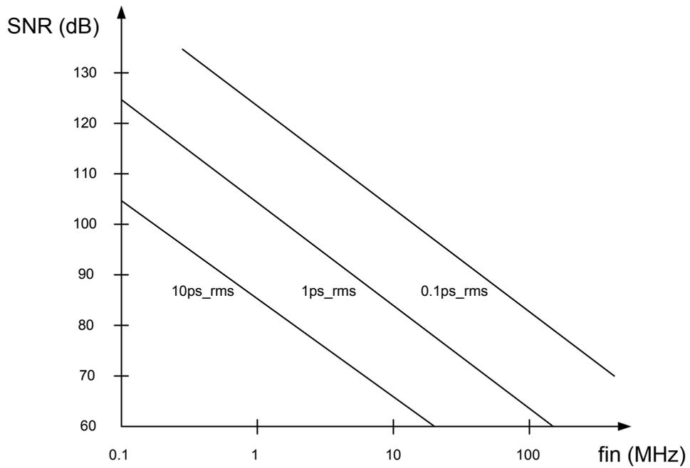
Figure 2.12: SNR due to jitter
