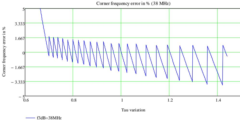
Figure 3.36: Cut off frequency error depending on the RC deviation at  $f_c=38\text{MHz}$
