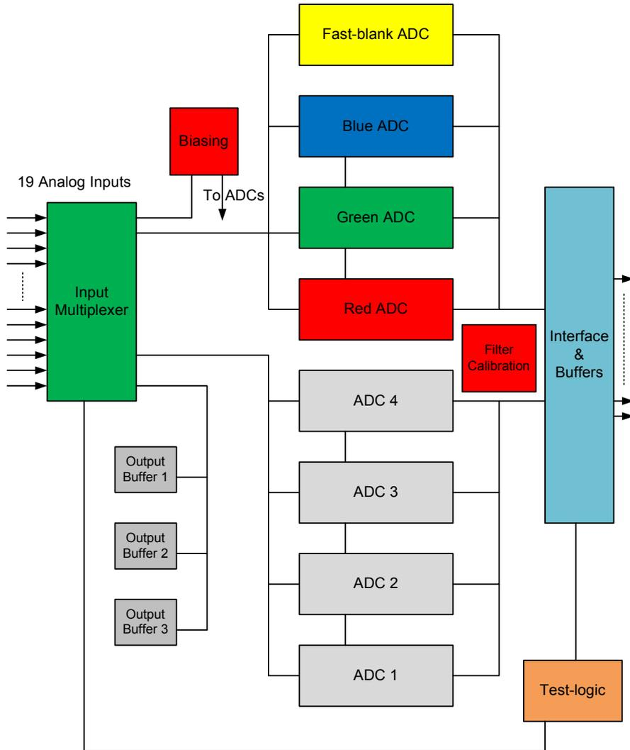
Figure 6.1: Principle top-level of the whole analog video frontend
