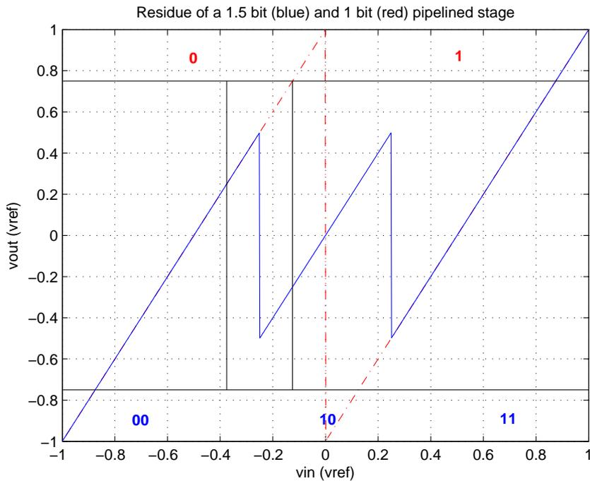
Figure 2.14: Residue of 1 bit and 1.5bit stage
