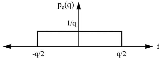
Figure 2.8: Equally distributed quantization noise
