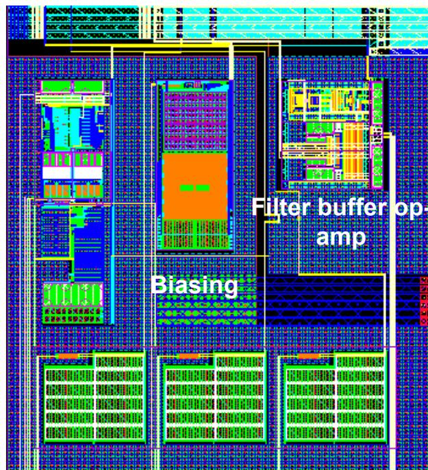
Figure 3.44: Layout of the filter buffer of the 65nm test-chip
