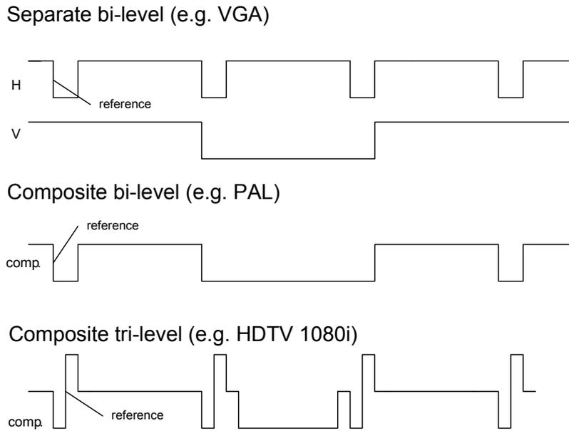
Figure 2.4: Synchronization depending on the TV system
