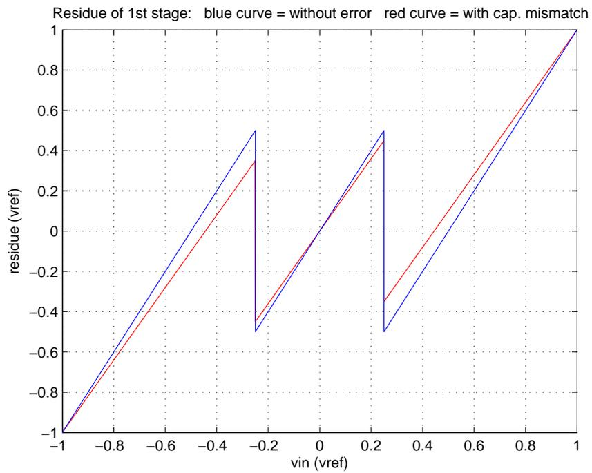
Figure 2.18: Residue of a 1.5bit stage with capacitor mismatch
