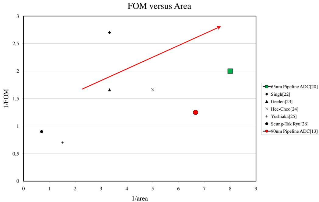
Figure 5.11: 1/FOM versus 1/area of the 65nm and 90nm pipeline ADC compared to state of the art ADCs
