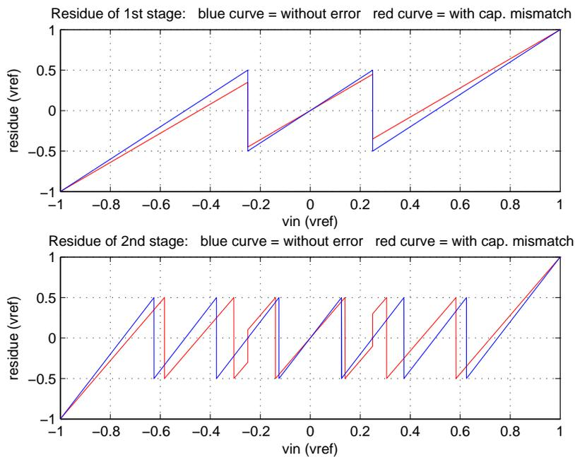
Figure 2.20: Residue of the first and second 1.5bit stage with capacitor mismatch
