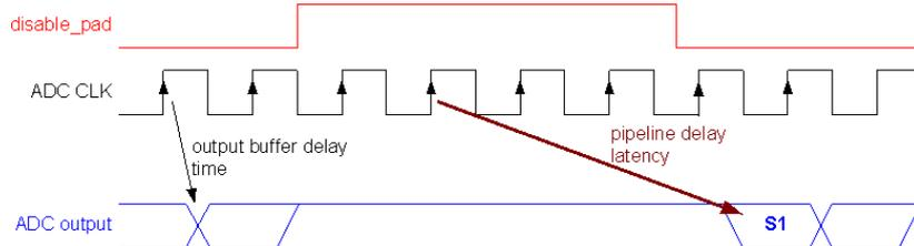
Figure 4.9: ADC output signal gating
