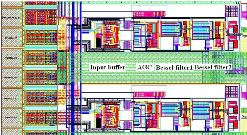
Figure 3.38: Layout of the two pre-processing's of the 90nm test-chip
