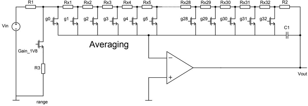
Figure 3.18: Simplified topology of the AGC with tapped resistor
