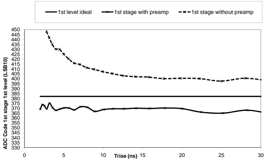
Figure 5.5: Sub-ADC output of the first stage with and without a preamp related to the ADC output measured with an input step of 0.8Vpp at 20MHz fstroke
