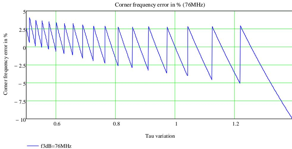
Figure 3.37: Cut off frequency error depending on the RC deviation at  $f_c=76\text{MHz}$
