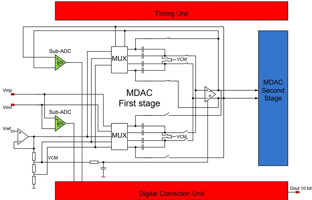
Figure 4.2: MDAC of the first stage with op-amp sharing
