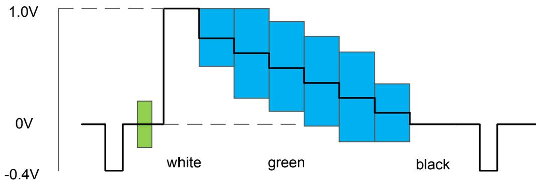
Figure 3.8: Standard video signal with synchronization pulse und black porch
