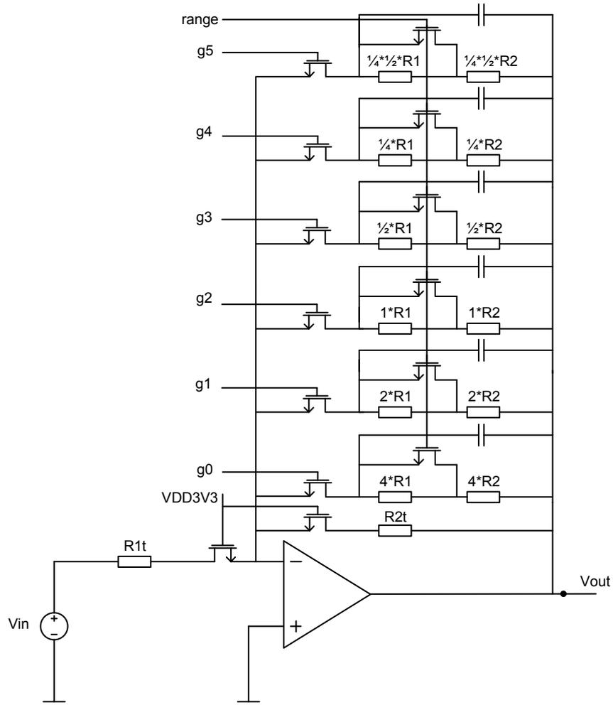
Figure 3.11: Principle topology of the AGC with binary weighted resistors in the feedback path
