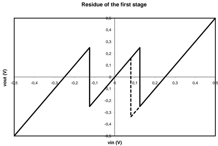
Figure 5.4: Residue of the first stage. The dotted line corresponds to an aperture error due to different sample times of MDAC and sub-ADC
