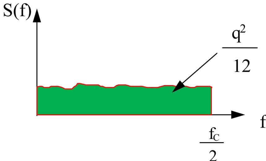
Figure 2.9: Noise density spectrum of the quantization noise
