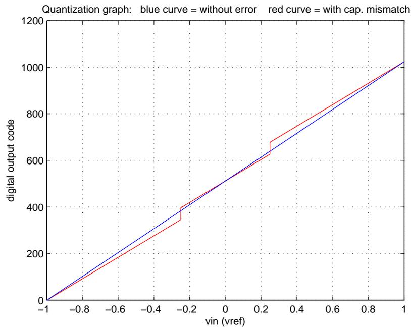
Figure 2.19: Residue of the first and second 1.5bit stage with capacitor mismatch
