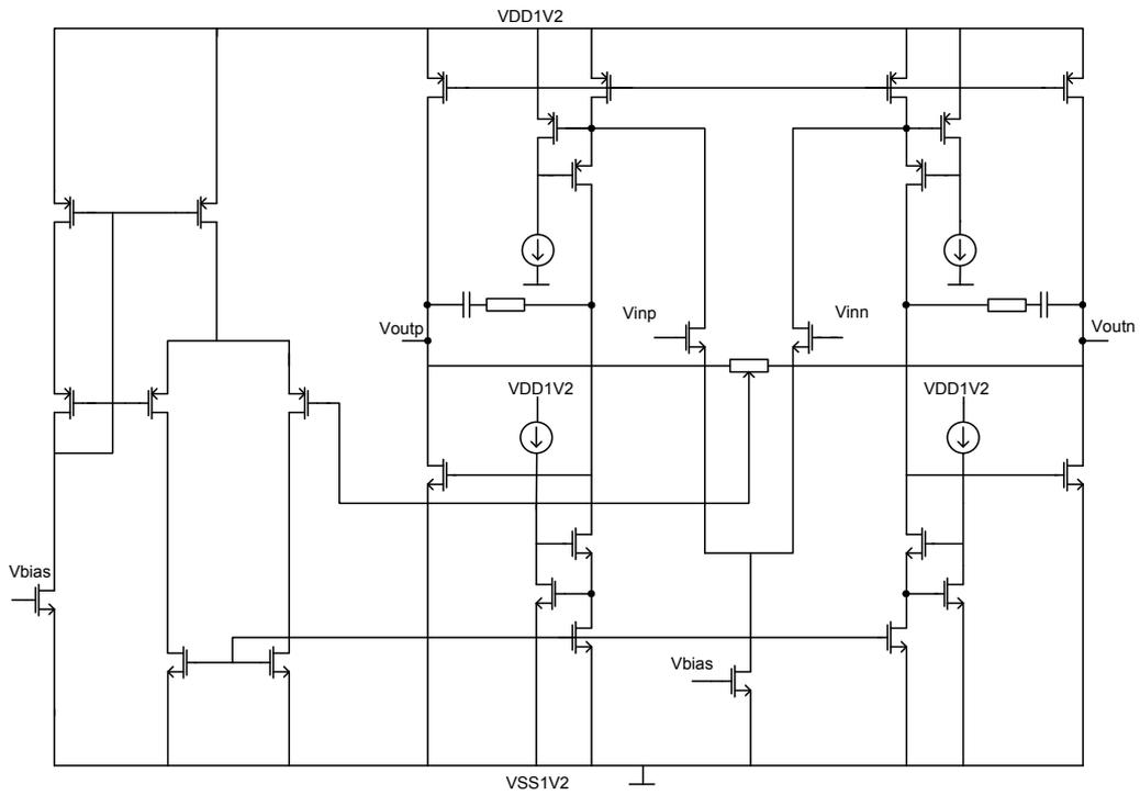
Figure 4.6: MDAC folded cascode op-amp Miller compensation
