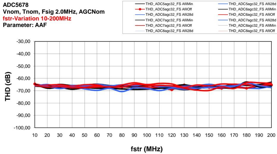
Figure 6.5: THD of the HD channels depending on fstroke
