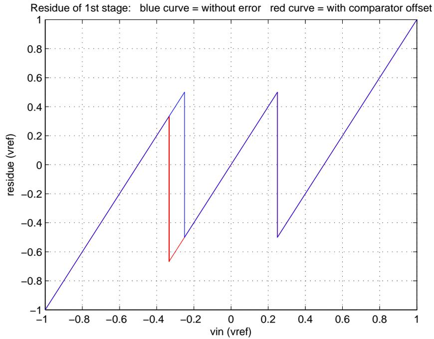
Figure 2.15: Residue of a 1.5bit stage with comparator offset
