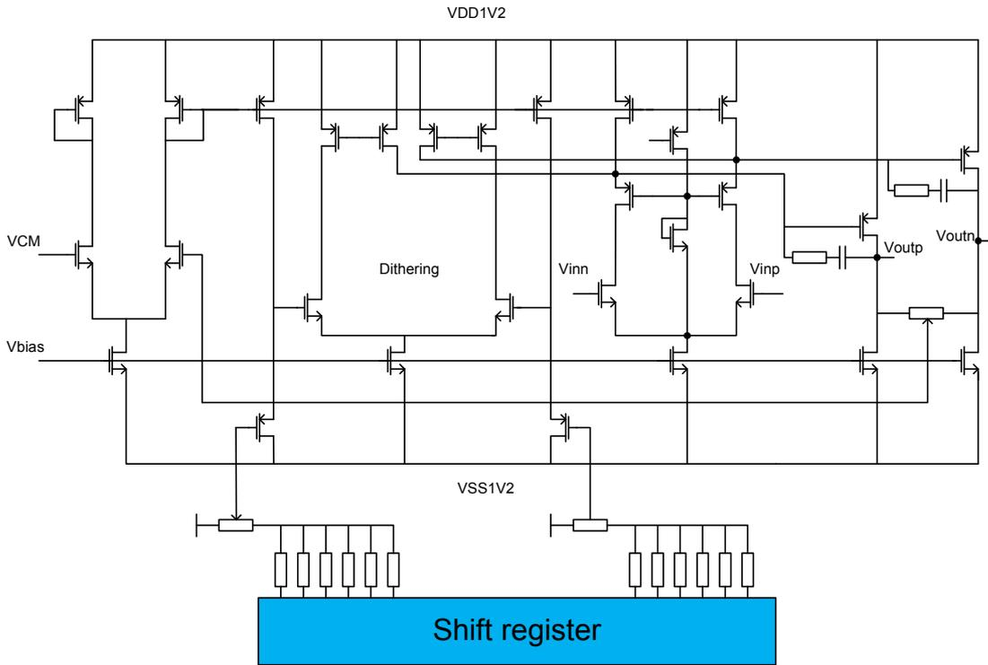
Figure 3.30: Op-amp of the second filter stage
