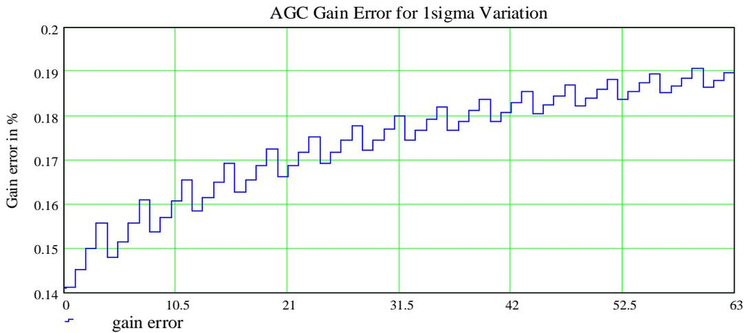
Figure 3.14: Gain error in % for one sigma variation of the resistors for 65nm technology
