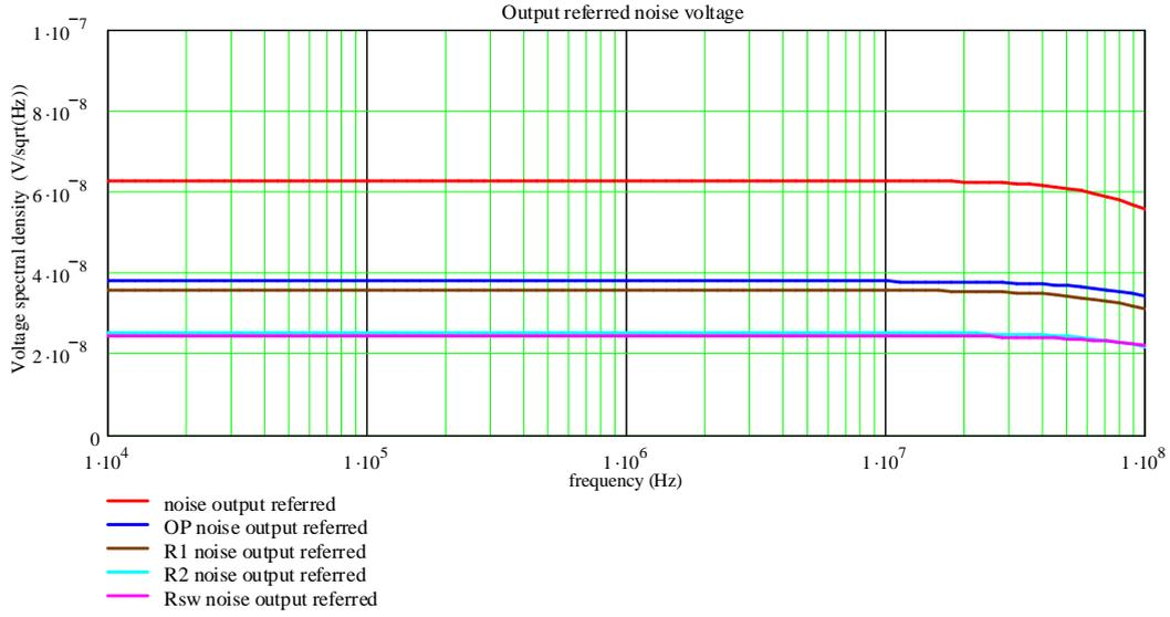
Figure 3.19: Noise of the different resistors at the output of the AGC
