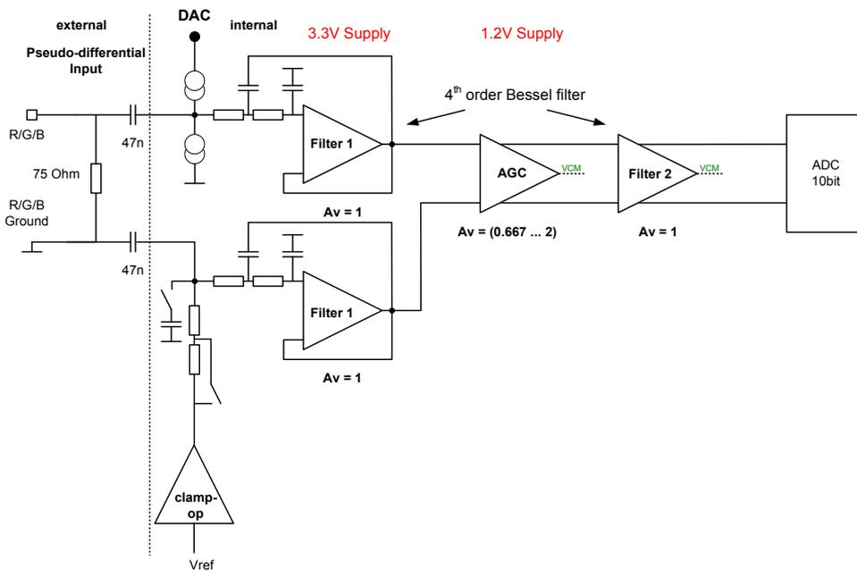
Figure 3.2: Principle Analog video Frontend with a 4<sup>th</sup> order Bessel filter using a Sallen-Key input stage
