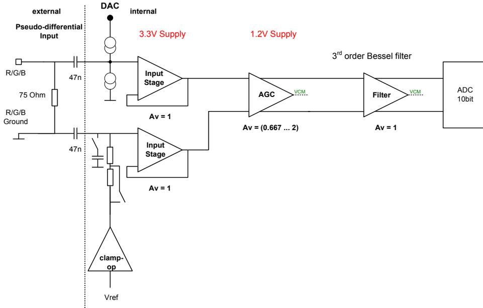
Figure 3.3: Principle Analog video Frontend with a 3<sup>rd</sup> order Bessel filter
