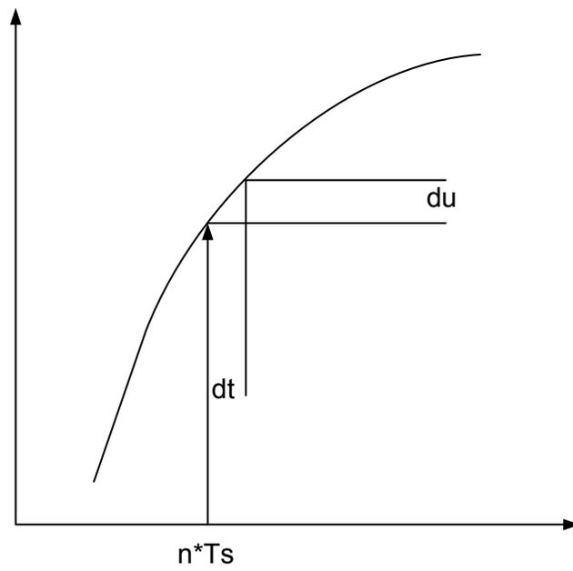
Figure 2.11: Jitter at the sampling process
