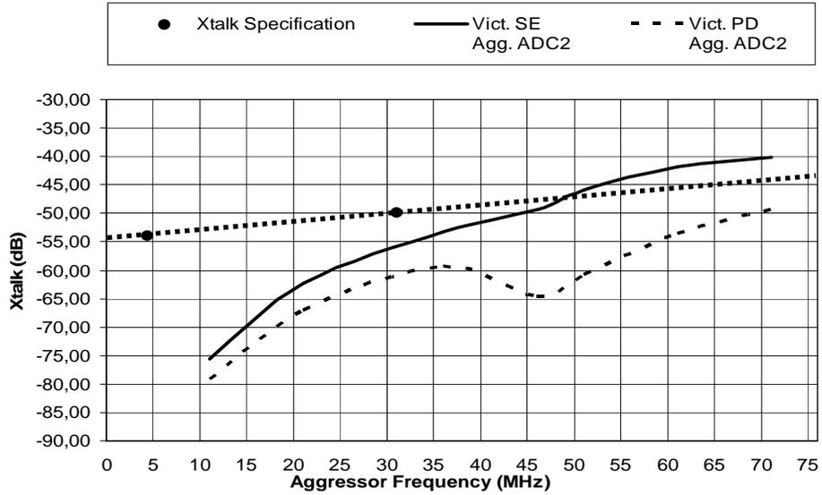
Figure 3.39: Crosstalk from pre-processing2 to ADC1 with and without pseudo differential input
