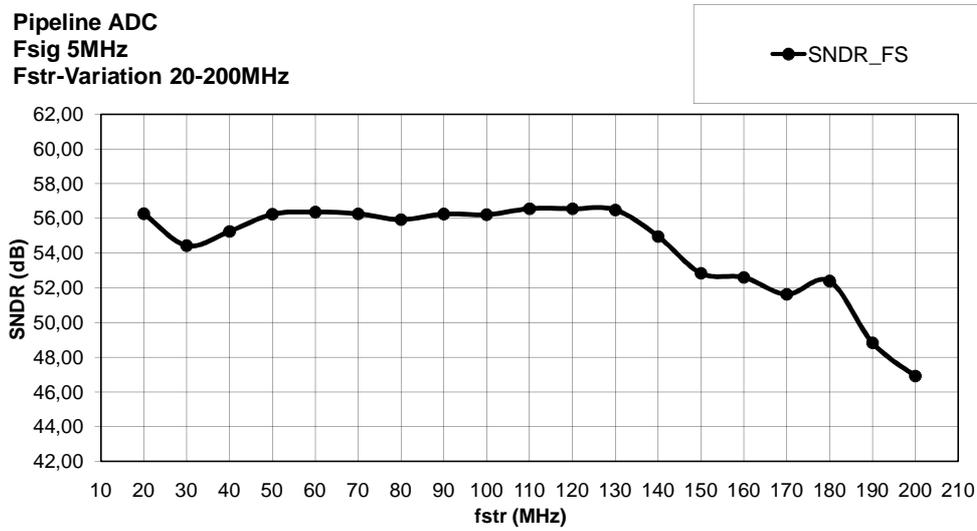
Figure 5.8: Signal to noise and distortion ratio depending on the strobe frequency
