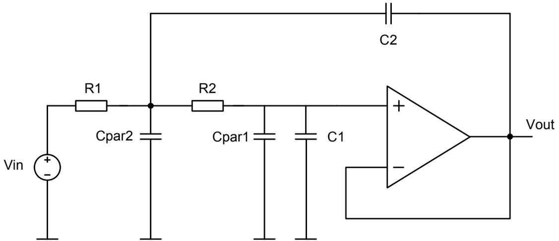
Figure 3.6: Principle topology of the Sallen Key filter
