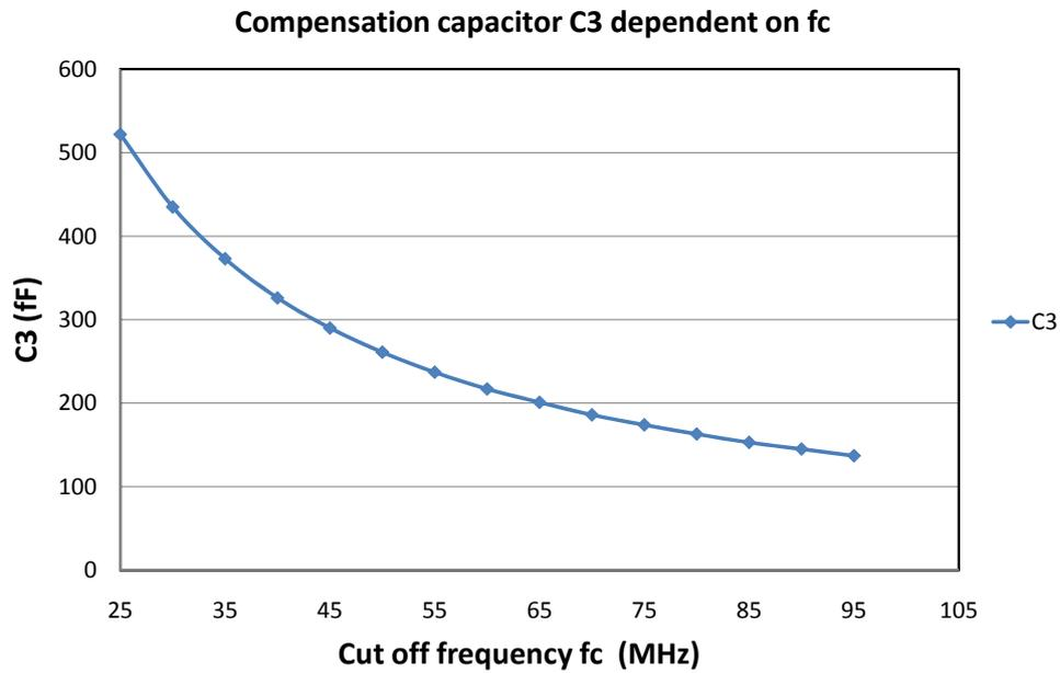
Figure 3.16: Calculation of the compensation capacitor  $C_3$  depending on the cut off frequency
