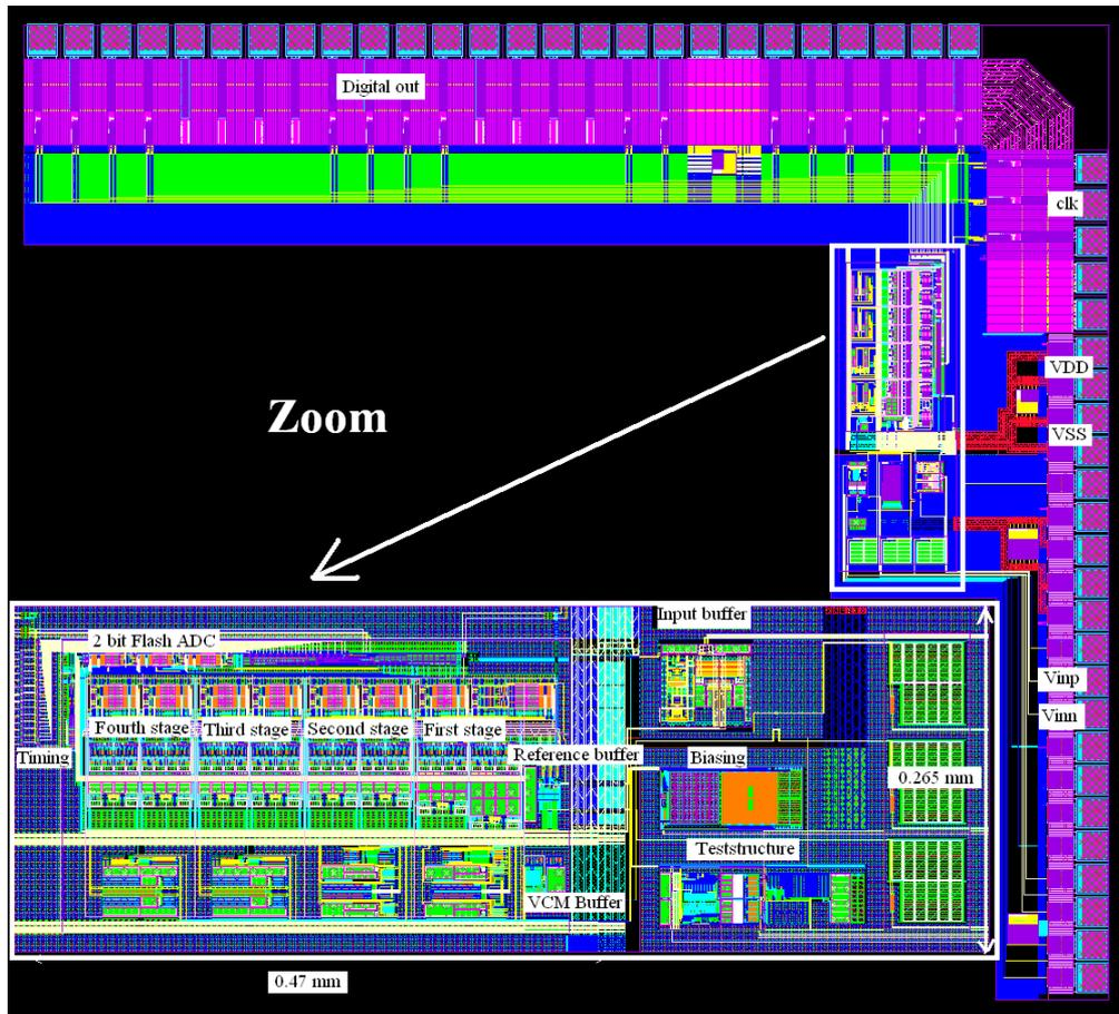
Figure 5.7: ADC and test-chip layout
