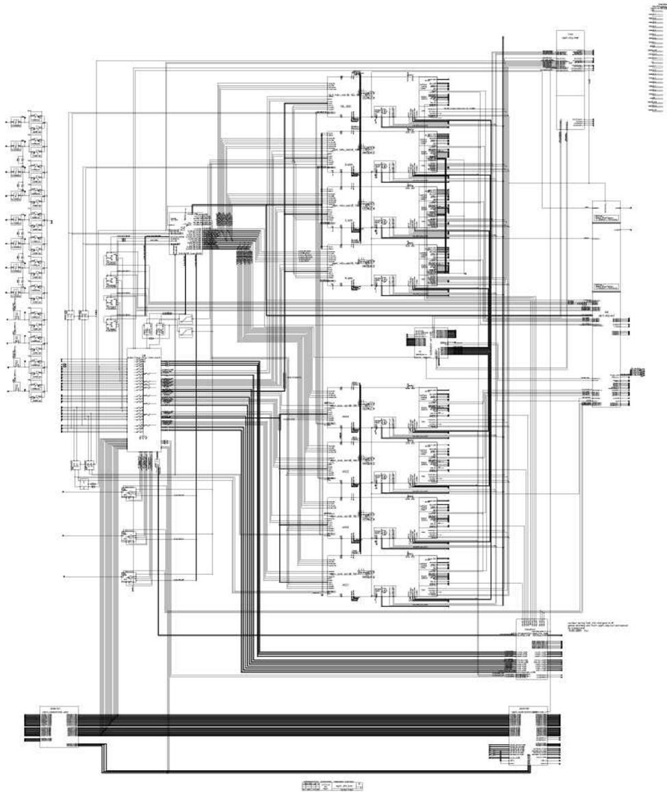
Figure 6.2: Top-level schematic of the whole analog video frontend
