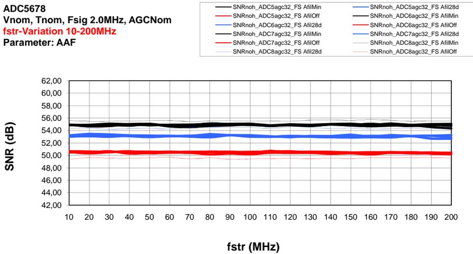
Figure 6.4: SNR of the HD channels depending on fstroke
