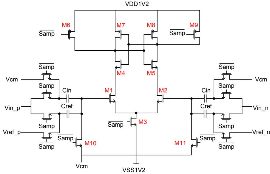
Figure 4.4: Comparator for the sub-ADC
