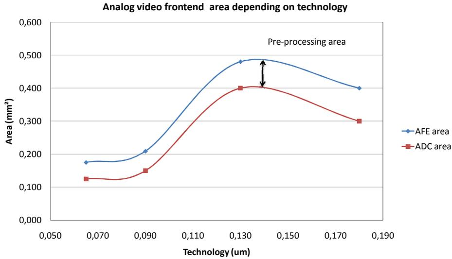
Figure 1.3: Analog video frontend area depending on technology
