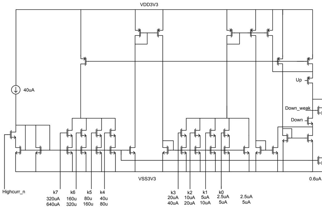
Figure 3.9: Principle schematic of the current steering clamp DAC
