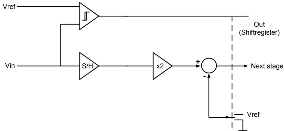
Figure 2.13: Pipeline ADC principle
