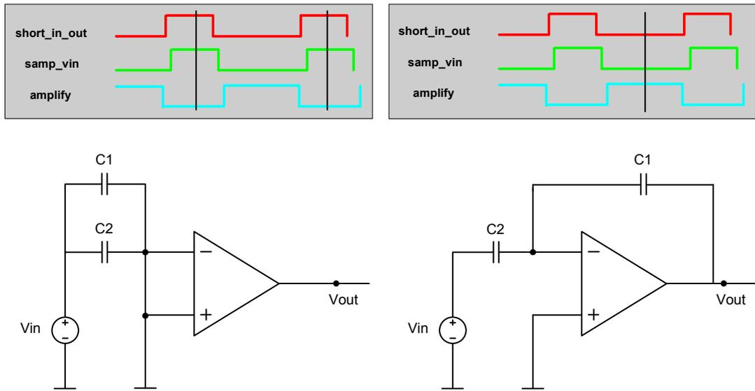
Figure 2.17: MDAC op-amp in sampling and amplification mode
