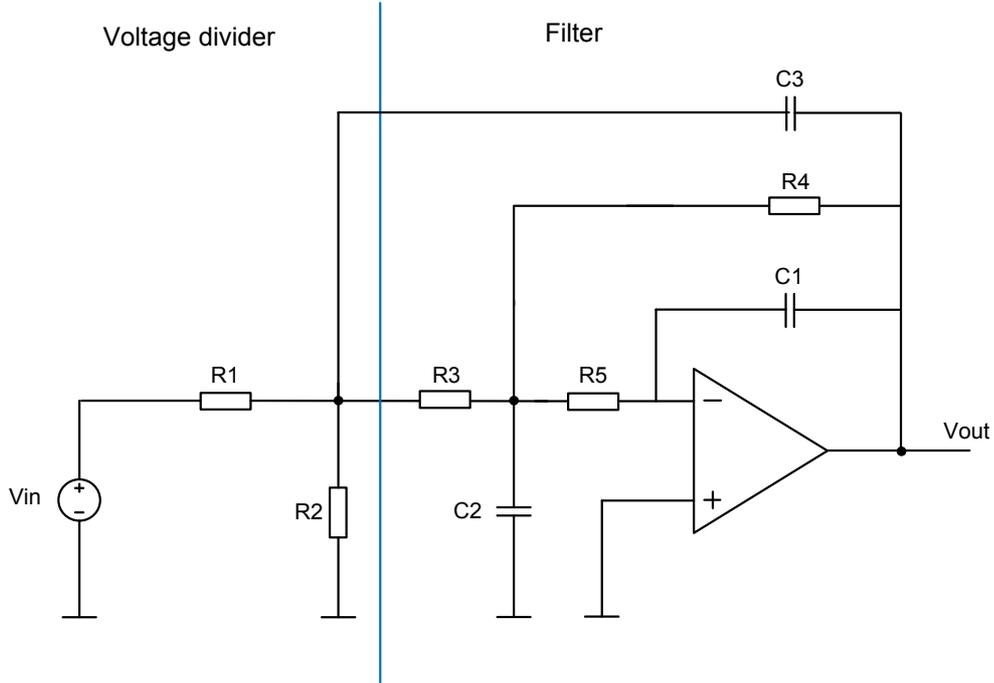
Figure 3.15: Simplified topology of the AGC with T-network in the input branch
