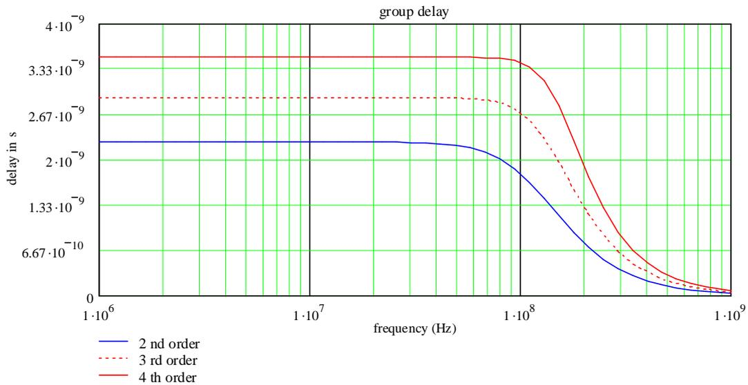
Figure 3.25: Comparison of the different group delays depending on the Bessel filter orders
