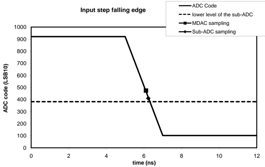
Figure 5.3: Input step at the output of the ADC with different sample points of the MDAC and the sub-ADC
