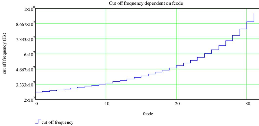
Figure 3.35: Cut off frequency of the 5bit capacitor array depending on fcode
