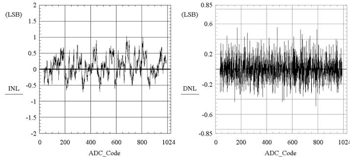
Figure 4.13: INL and DNL fsig=2MHz at fs=165MS/s
