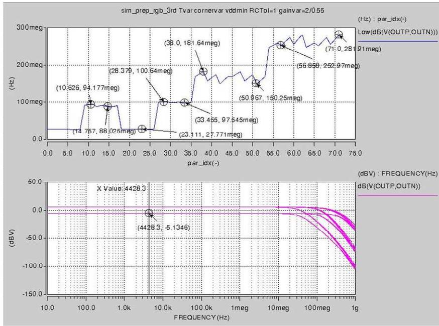
Figure 3.45: Variation of the cut off frequencies depending on the process corner
