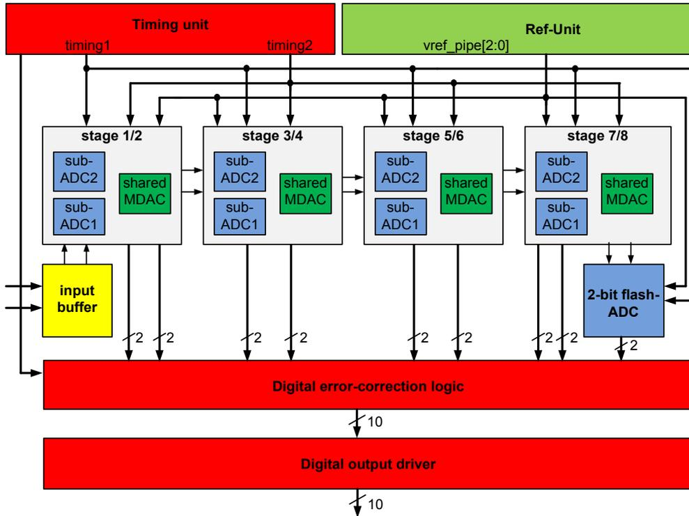
Figure 4.1: Principle architecture of the 90nm pipeline ADC
