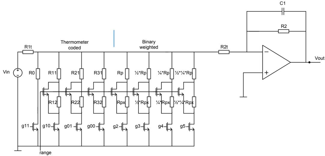
Figure 3.13: Principle topology of the AGC with binary weighted resistors in the input branch
