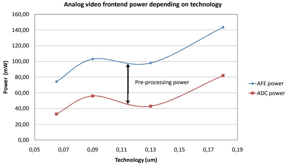
Figure 1.2: Analog video frontend power depending on technology
