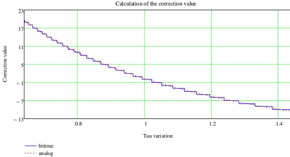
Figure 3.34: Calculation of the correction value depending on the RC deviation at fcode 7
