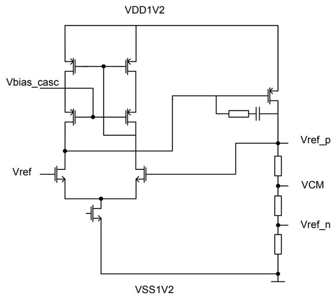
Figure 4.7: Single ended reference buffer
