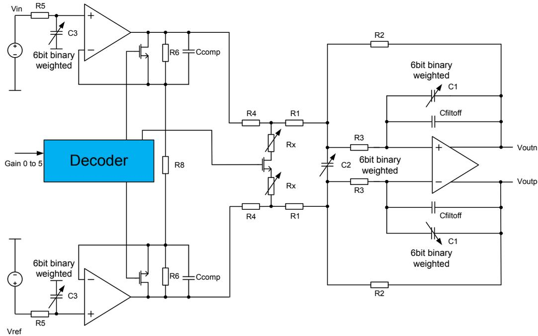
Figure 3.22: Low noise 2 stage 3<sup>rd</sup> order pre-processing
