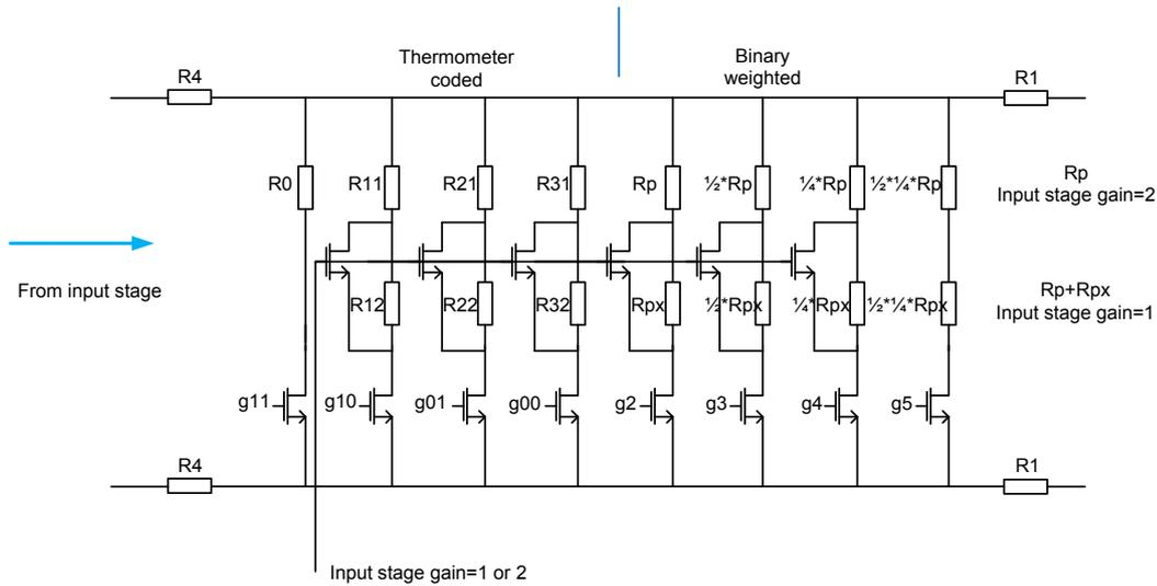
Figure 3.23: T-network of the low noise 2 stage 3<sup>rd</sup> order pre-processing
