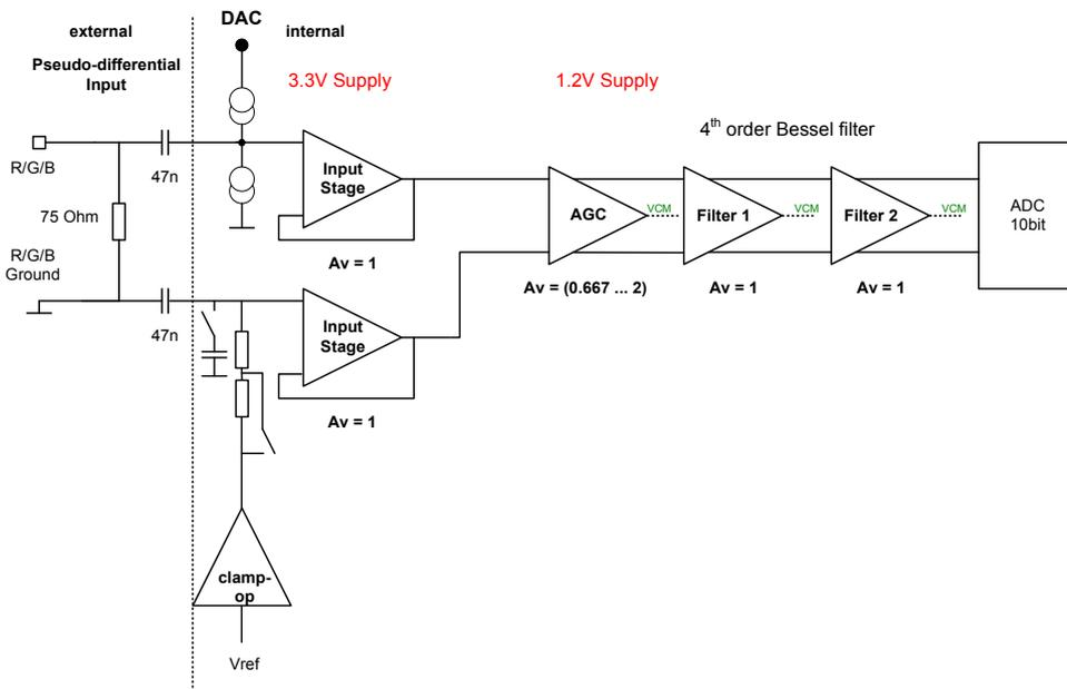
Figure 3.1: Principle Analog video Frontend with a 4<sup>th</sup> order Bessel filter
