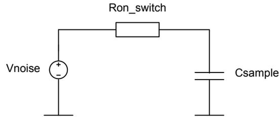
Figure 2.10: The equivalent circuit of a sample switch and capacitor
