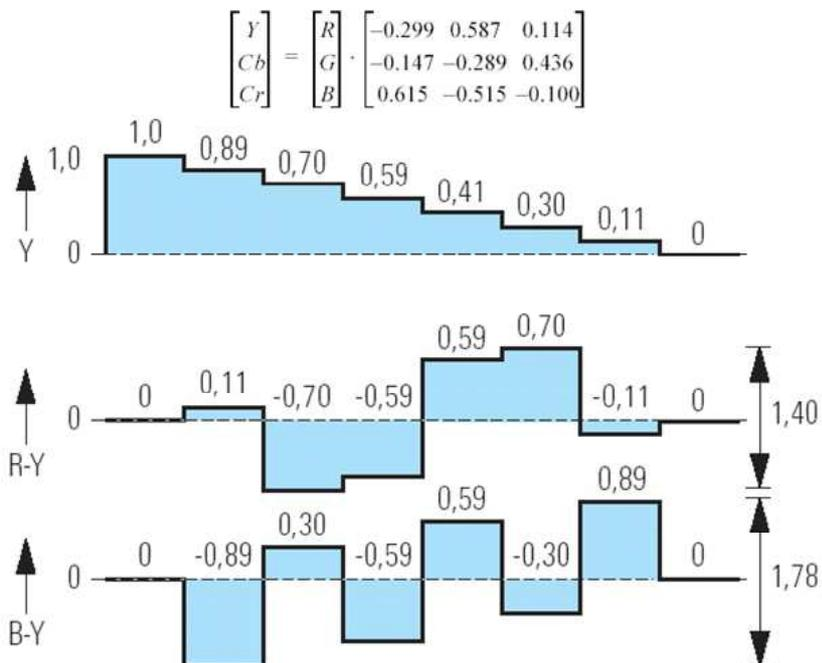
Figure 2.3: YUV signal with different color levels
