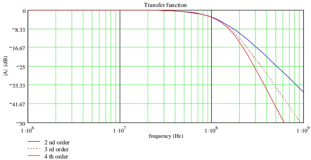
Figure 3.24: Comparison of the different Bessel filter orders for a cut off frequency of 96MHz
