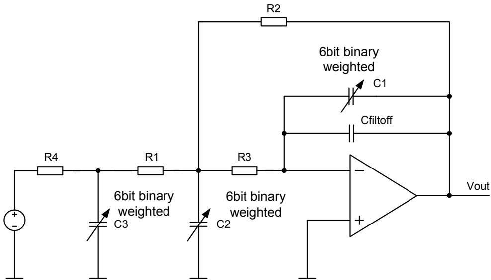
Figure 3.31: Combined topology of the 3<sup>rd</sup> order Bessel filter
