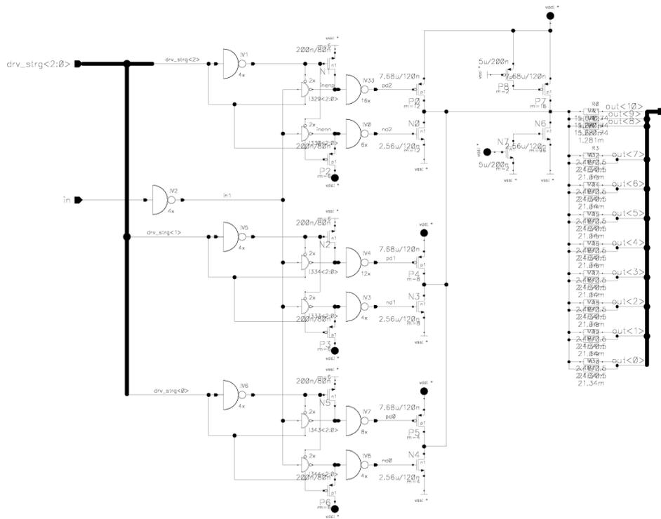
Figure 4.15: Schematic of the 1V digital output pad
