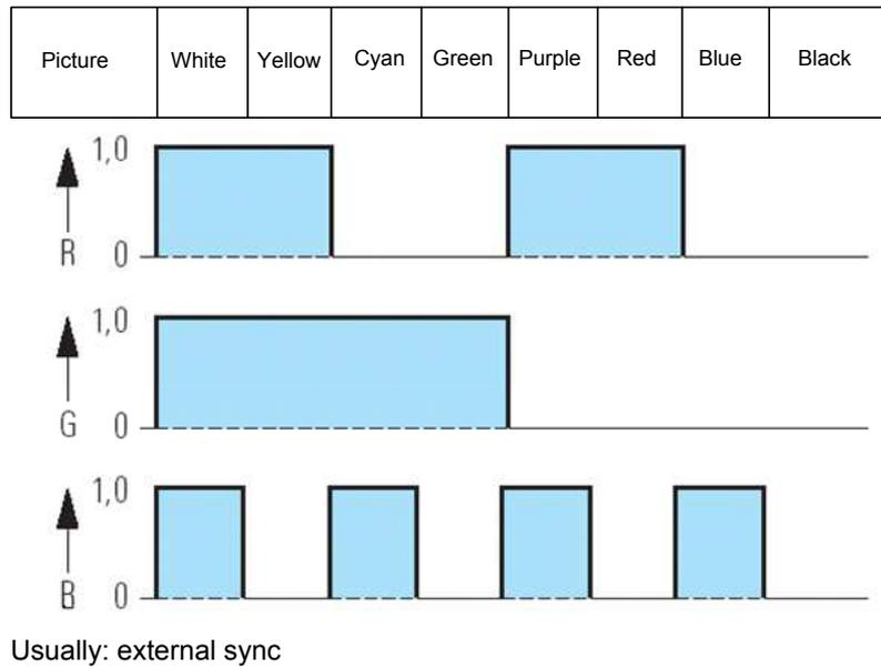
Figure 2.2: RGB signal with different color values
