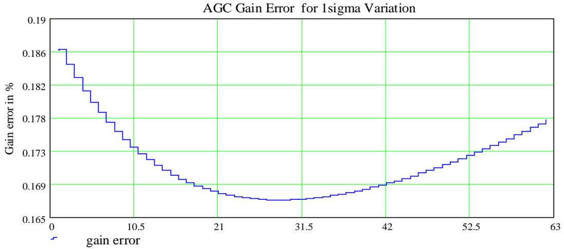
Figure 3.20: 1 sigma gain error of the AGC due to resistor mismatch for 65nm technology
