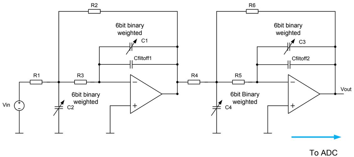
Figure 3.26: Topology of the 4<sup>th</sup> order Bessel filter
