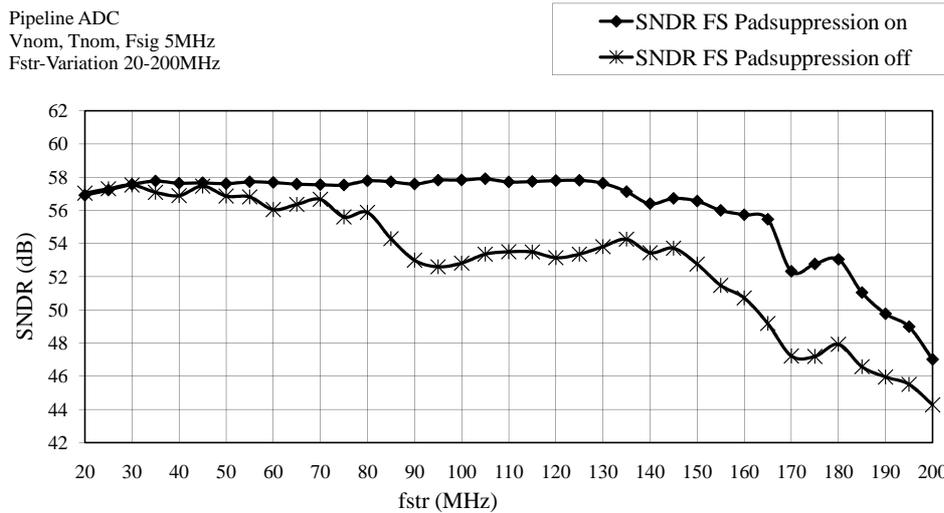
Figure 4.11: Signal to noise and distortion ratio with and without pad noise suppression technique
