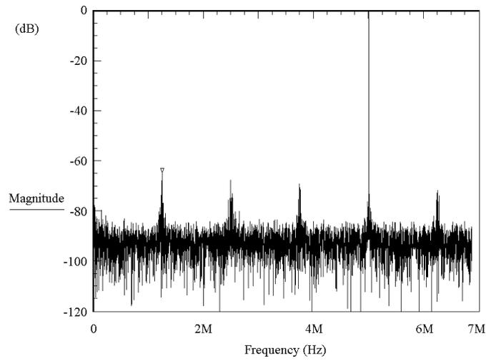
Figure 4.14: Decimated frequency spectrum at  $f_{sig}=60\text{MHz}$  and  $-2\text{dBFS}$
