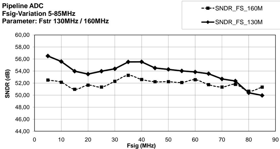
Figure 5.9: Signal to noise and distortion ratio depending on the signal frequency with 130 and 160 MHz fstroke
