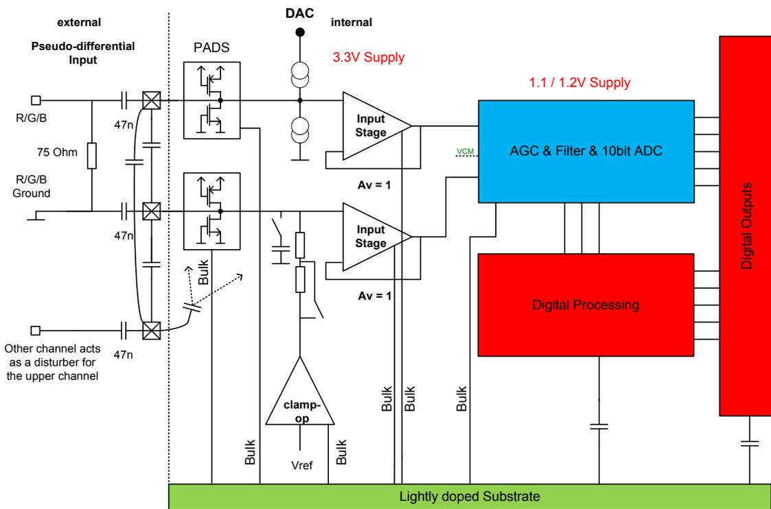
Figure 3.5: Principle topology of the pseudo differential input stage with its disturbance sources
