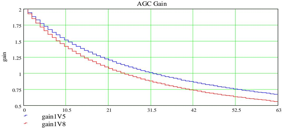
Figure 3.10: Characteristic of the AGC for two different input voltages
