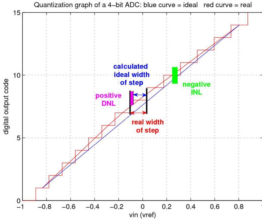
Figure 2.16: 4bit ADC characteristics with DNL and INL
