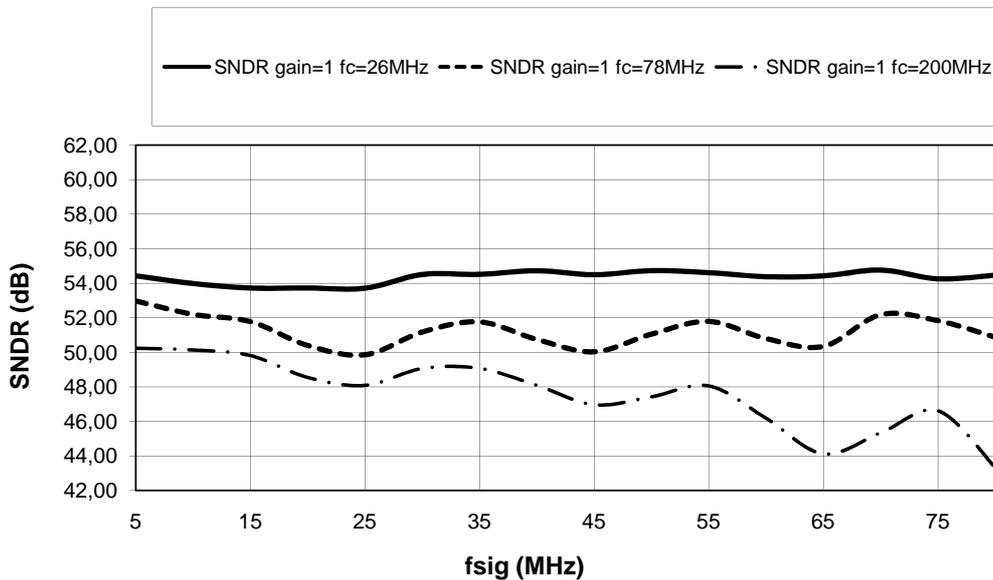
Figure 3.42: SNDR of the pre-processing at  $f_{stroke}=165\text{MHz}$  depending on the signal frequency
