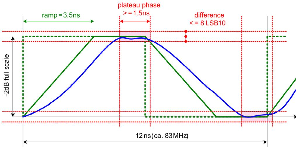
Figure 3.41: Specification of the step response for the filter off mode
