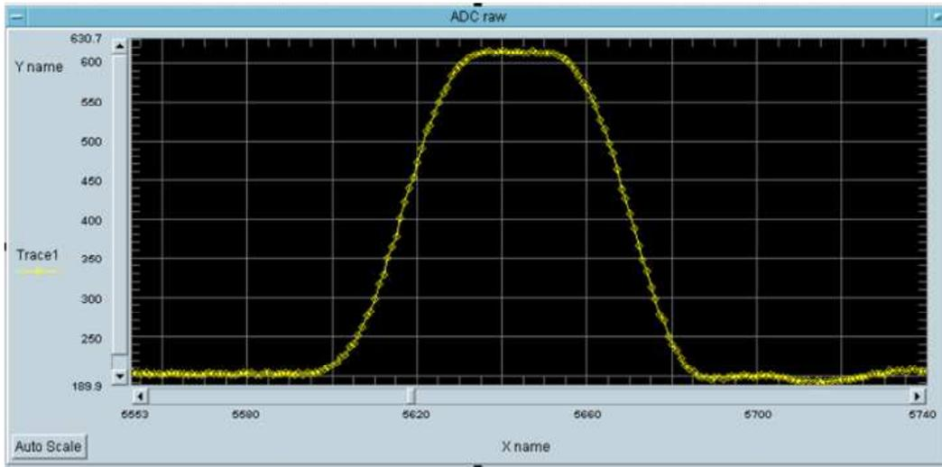
Figure 3.40: Step response of the pre-processing measured with a beat frequency test
