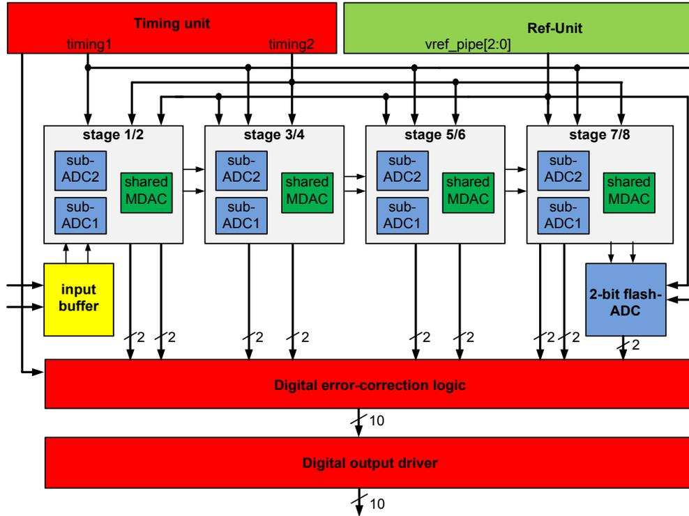
Figure 5.1: Principle architecture of the 65nm pipeline ADC
