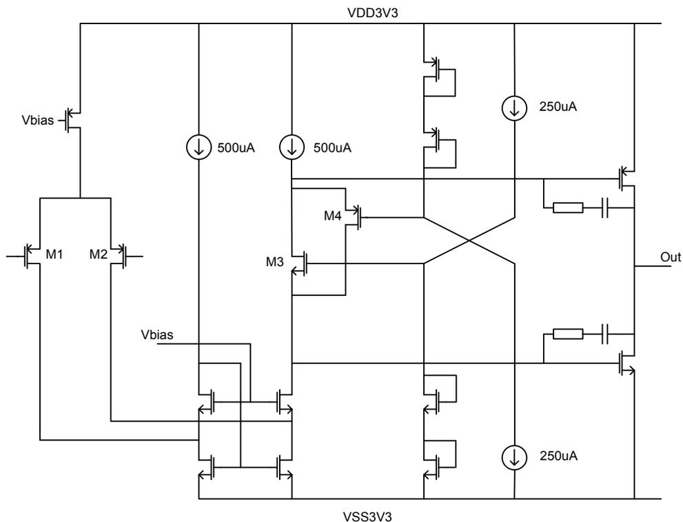
Figure 3.7: Principle schematic of the folded cascode class AB input buffer
