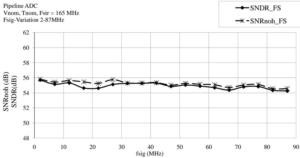
Figure 4.12: Signal to noise and distortion ratio depending on the signal frequency
