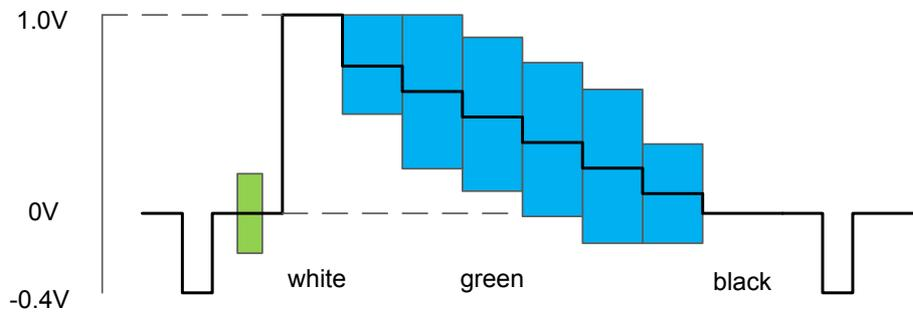
Figure 2.1: Composite signal with synchronization pulse and color burst
