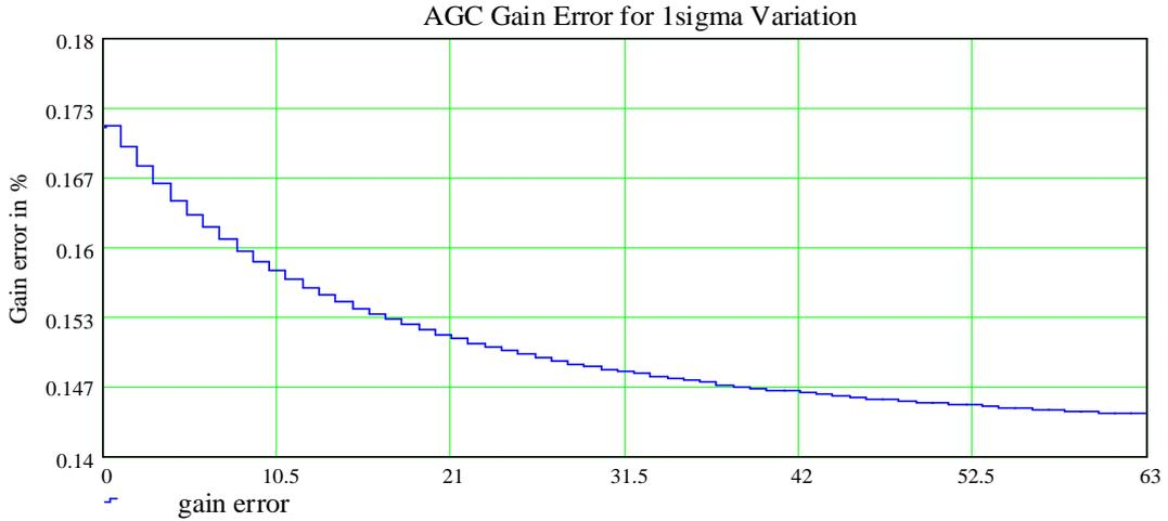
Figure 3.12: Gain error in % for one sigma variation of the resistors for 65nm technology
