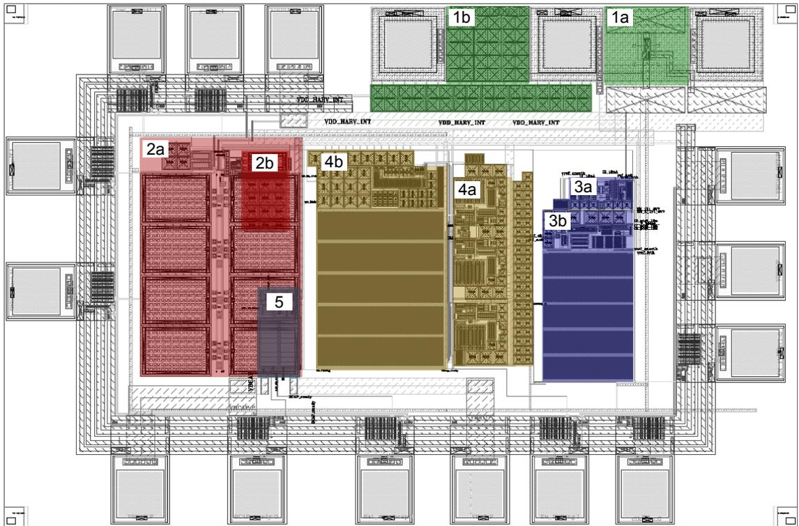
Figure A.1: Layout of the stand-alone version of the Electro-Magnetic Energy Harvester
