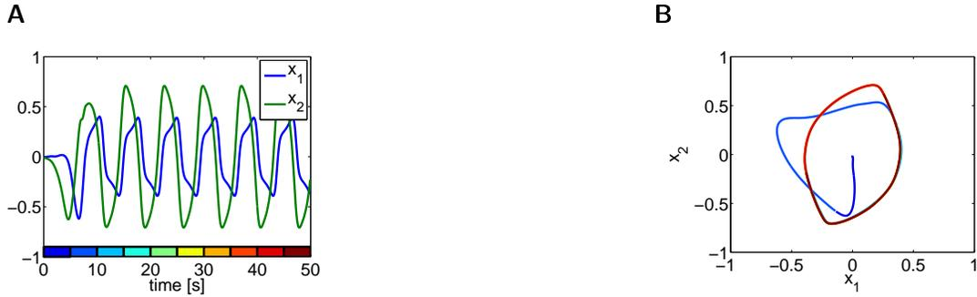
Figure 4.7: The swing up task. The network starts at rest and is able to swing itself up to its nominal limit cycle. Figure (A) shows the trajectories over time and (B) shows the same trajectories in phase plane. The color coding of (B) corresponds to the color labels of the time windows in (A).
