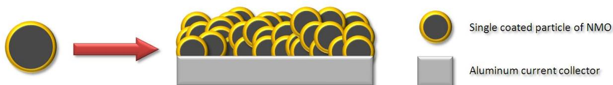
**Figure 60:** schematic illustration of the state of the art single particle coating of active materials like  $\text{Li}_{0.5}\text{Mn}_{1.5}\text{O}_4$ , which are prepared as electrodes after the coating process <sup>(source: author)</sup>.
