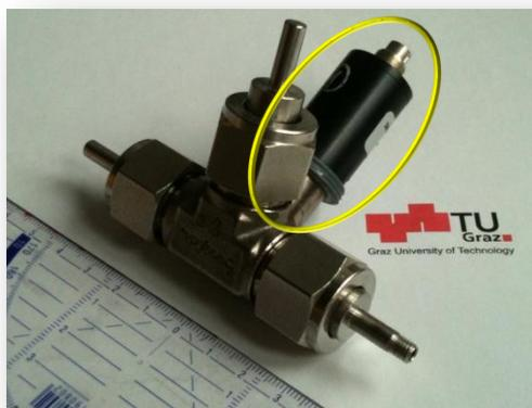
**Figure 90:** modified Swagelok®-cell; the yellow ellipse marks the pressure sensor <sup>(source: author)</sup>.
