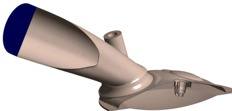
**Fig. 4.20:** Computational domain for the dynamic analysis of an intake port.
