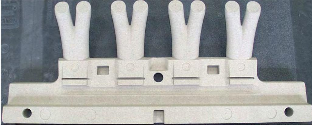
**Fig. 7.1:** Sand core for the tumble port of the eight-cylinder SI-engine.
