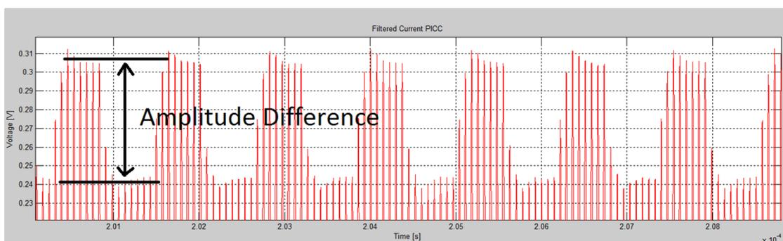
Figure 6.2: Amplitude difference of modulated current
