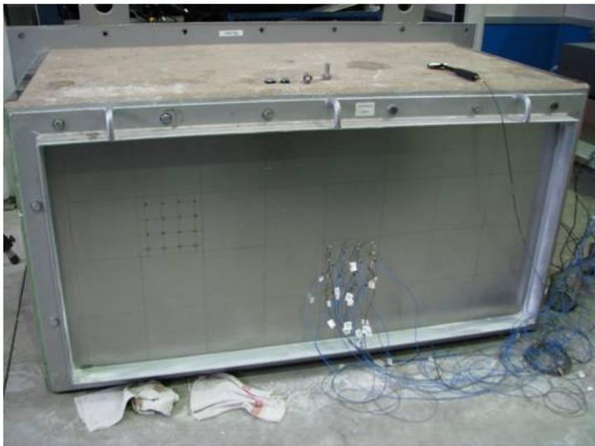
Figure 3.5: Front view of the test rig with the attached steel plate. For measurements of the component PTF of the plate, the opposite surface of the cavity can be removed
