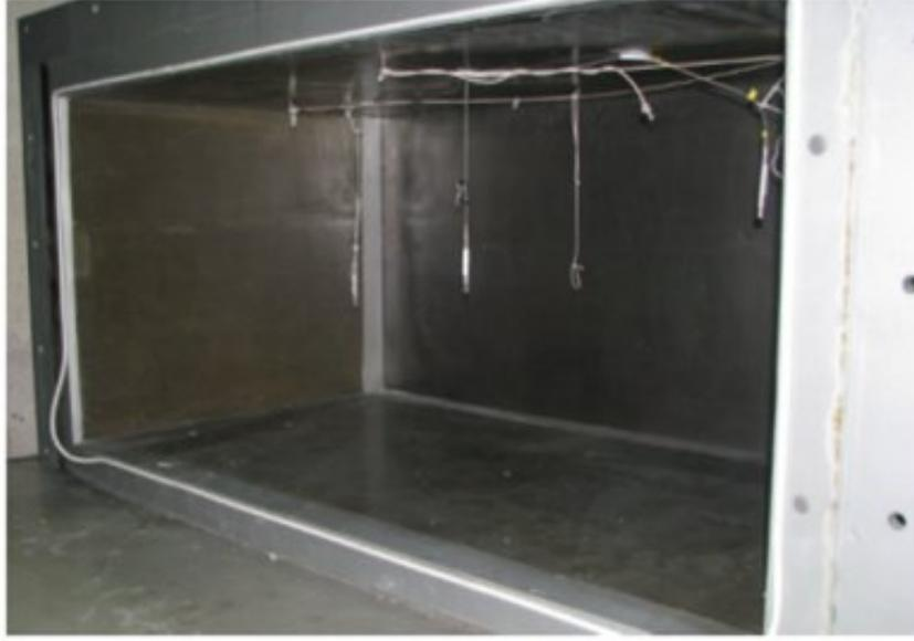
Figure 3.3: Interior of the air cavity for the PTF validation measurements. Microphones 1, 2 and 3 are visible.
