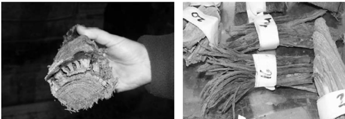
Figure 11: Oak (a) and alder (b) samples from the foundation of the Frari tower [from Bertolini et al. (2006)]
