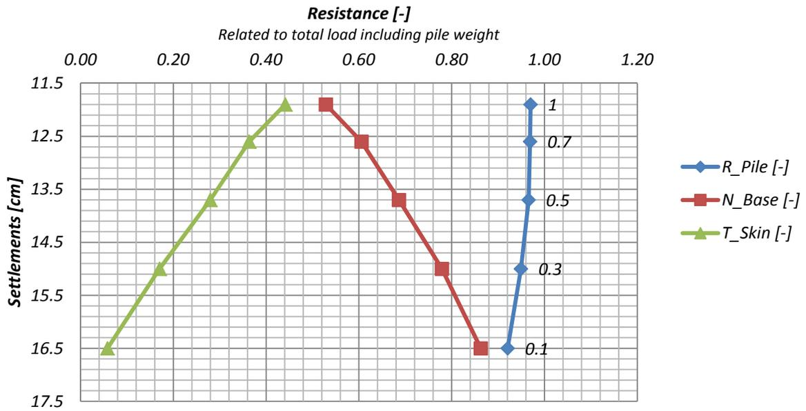
Figure 75: Resistance-settlement curve, Frari soil – HS model
