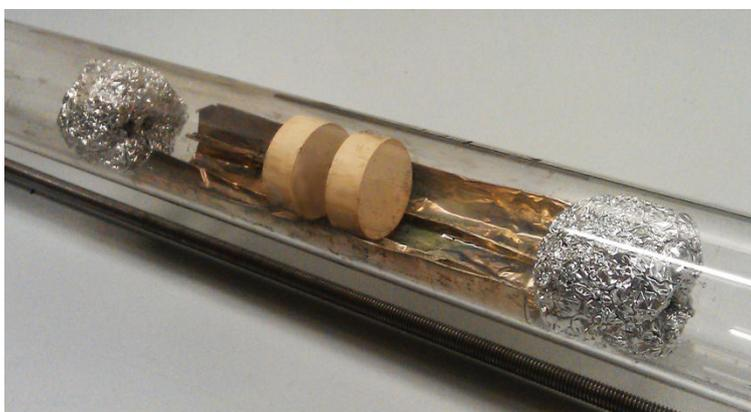
**Figure 43: Samples placed in glass tube with balls of aluminium foil placed before and after the vessel**
