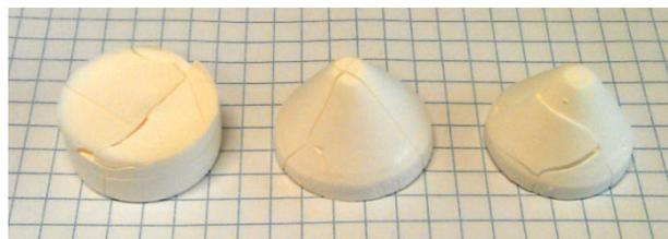
Figure 18: Examples of specimens cracked after swelling. The grid size is 5 mm.
