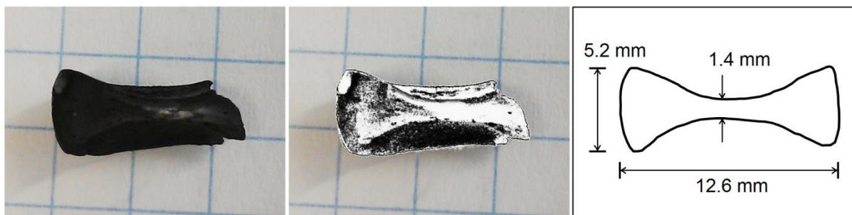
**Figure 36: Sample H40\_II broken in half after carbonisation at 900°C, grid size is 5 mm; left: original image; middle: enhanced image of left frame; right: contours of sample's cross-section with measurements**
