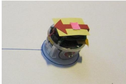
**Figure 12: The e-puck is a small robot, which can move through two independently controlled wheels. The figure shows the robot that was used in the presented experiments. The red arrow informs the user about the current direction of the robot. For tracking purposes, the pink square was placed on the center of the e-puck.**
