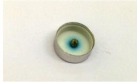
Figure 40: Nickel sample showing oxidation after being exposed to its melting temperature several times using the DSC 404 C
