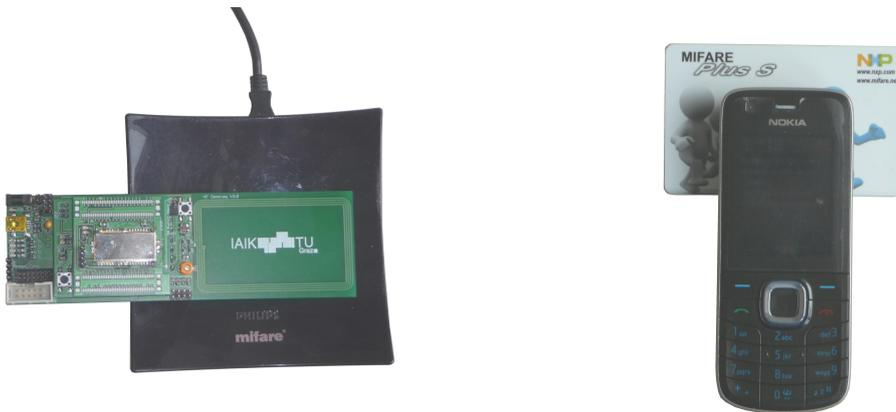
(a) Picture of the PCD with the proxy in range.
