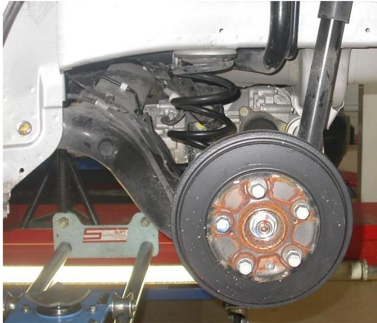
**Figure 4.13 Suzuki SX4 rear suspension [MAG06]**
