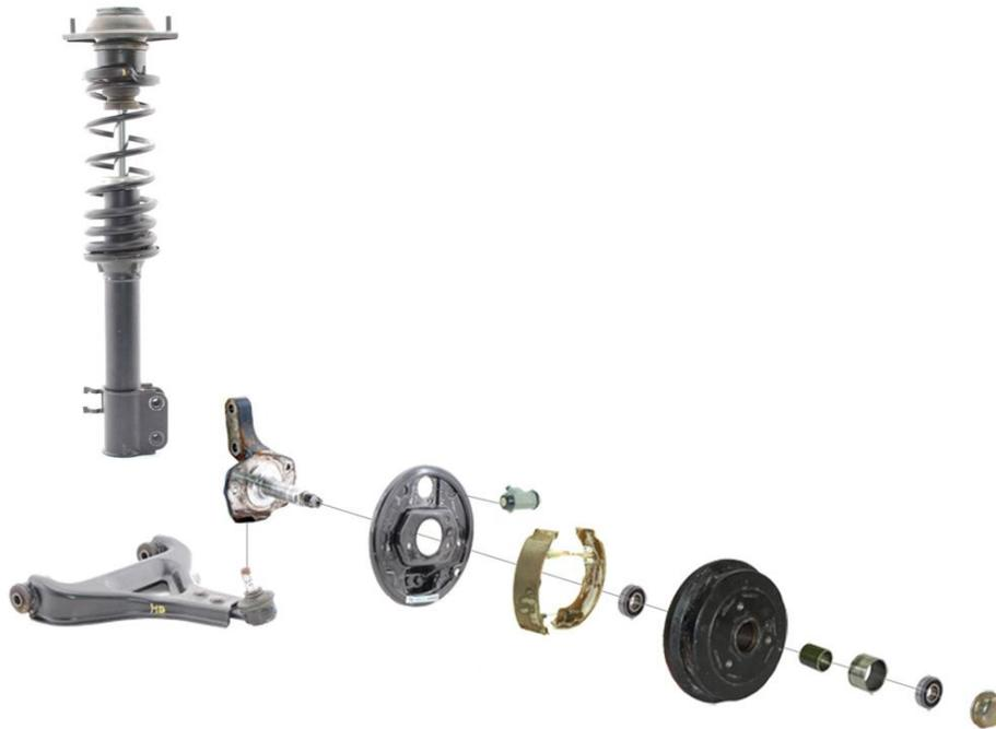
**Figure 4.8 Tata Nano front suspension without steering [A2M10]**
