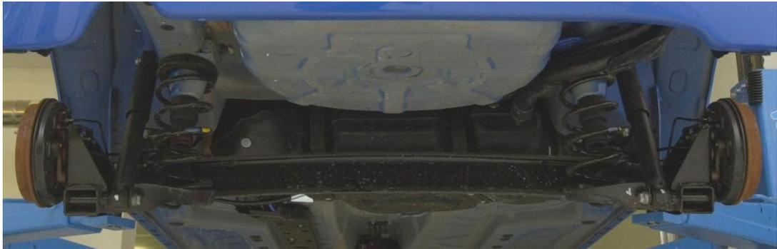
***Figure 4.15 Fiat Panda twist beam suspension [A2M10]***
