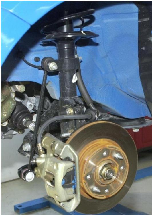
**Figure 4.5 Fiat Panda front suspension [A2M10]**
