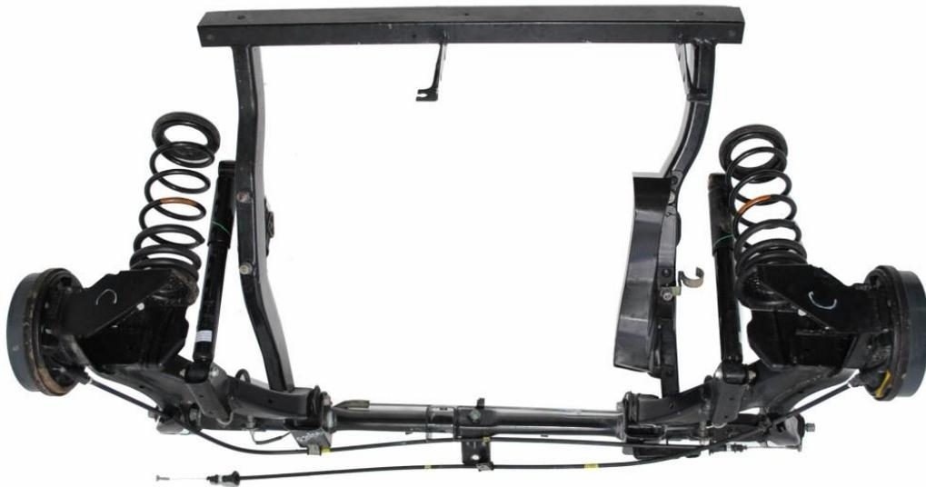
**Figure 4.16 Tata Nano semi trailing arm suspension with subframe [A2M10]**
