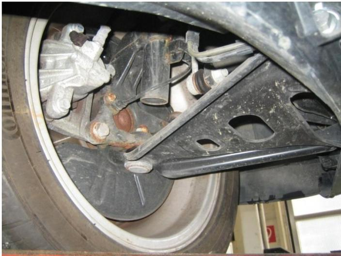
**Figure 4.4 SMART Fortwo II steering knuckle and wishbone**
