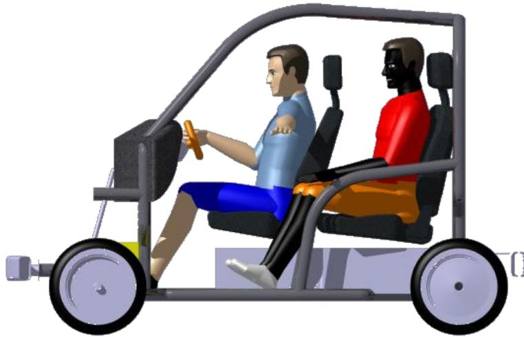
**Figure 2.1 First vehicle layout – sideview [PSM09]**
