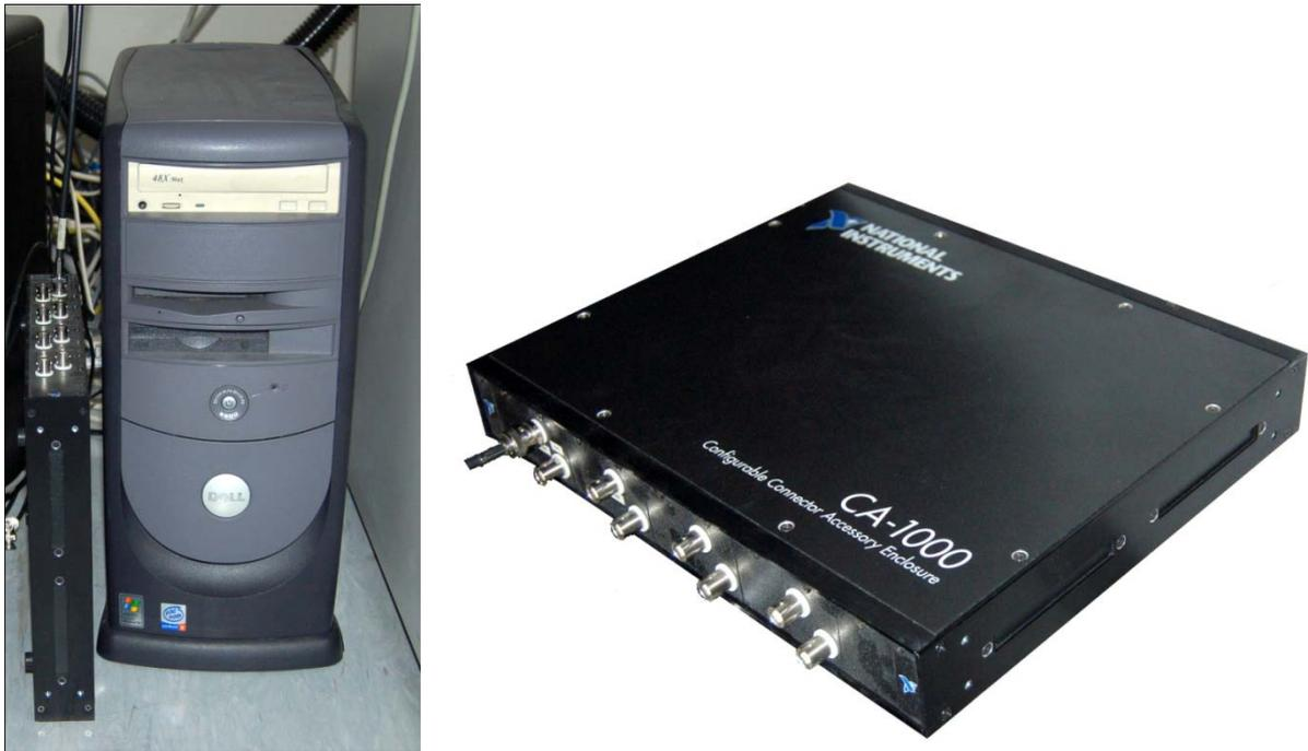
Figure 3-21: In the left image the analyzing PC with the ADC card is shown. The right image shows the used ADC card adapter.
