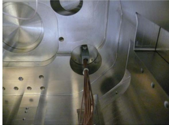
Figure 3-18: Shows the cable which gets through a RS232 flange out of the FIB.
