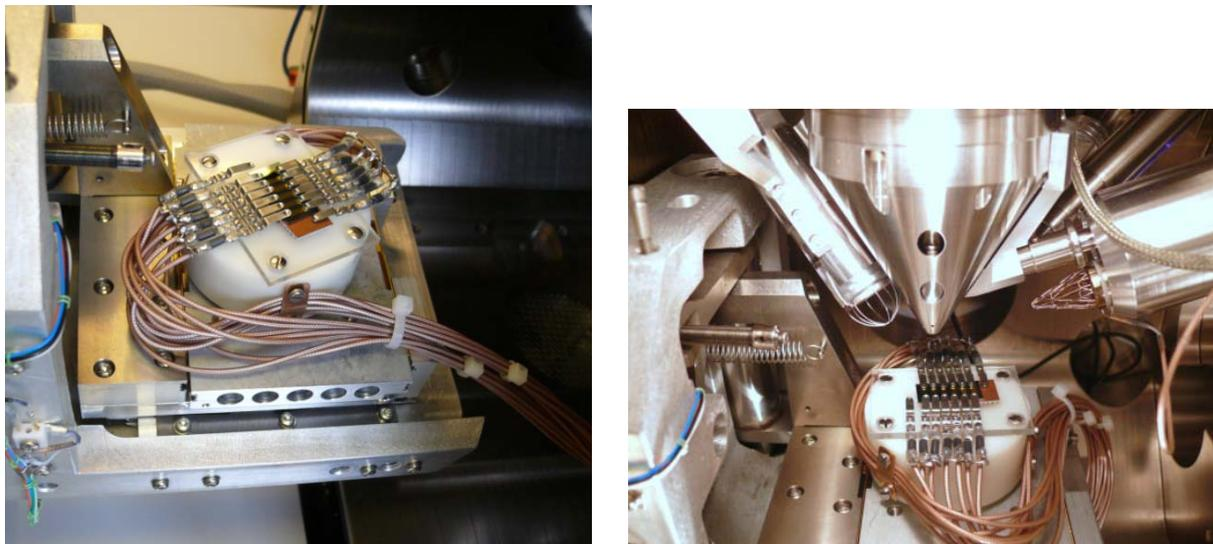
Figure 3-19: The left image shows the specimen holder which is build in the FIB while the chamber is open whereas the right image shows it while the chamber is closed. In both cases the mounted specimen is the second prototype.
